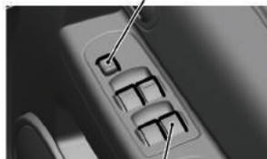
Fuel tank filler door release lever
