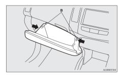
4. Remove the lower glove box fastener, and then remove the lower glove box.
