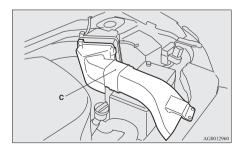
4. Remove the duct (C) after removing the air cleaner filter (D).
