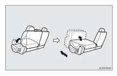
On vehicles without second seat slide function, the seatbacks fold forward. Lift the entire seat unit until you hear a click.
