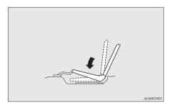
6. Fold the seatback while pulling the belt (F) located in the centre of the seatback.
