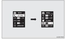
Press and hold the multi-information meter switch for about 2 seconds or more to switch in sequence from 1 (turn-signal sound 1) → 2 (turn-signal sound 2) → 1 (turn-signal sound 1).
