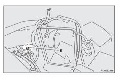
6. Loosen the plug (G) at the fuel filter (E) with the hexagonal wrench (5 mm).
