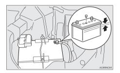
The electrolyte level must be between the specified limit on the outside of the battery. Replenish with distilled water as necessary.
