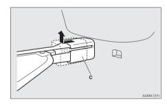
To fit the cargo area cover, follow the removal steps in reverse. Gently shake the entire cargo area cover after fitting it to make sure it is securely retained.
