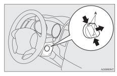
Insert the emergency key into the ignition switch.
