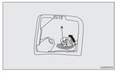
4. Remove the bulb from the socket.
