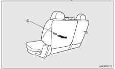
On vehicles with second seat slide function, the seatbacks fold forward, and then the entire seat unit rises up while moving forward.
