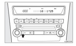
Push the CD button (2) if a disc is already in the CD player. The audio system will enter CD mode and start playback. The track number and the playing-time will appear on the display. The tracks in the disc will be played consecutively and continuously.
