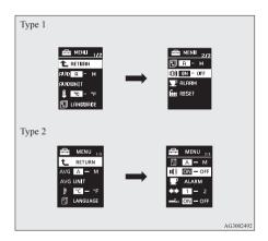
Press and hold the multi-information meter switch for about 2 seconds or more to switch in sequence from ON (operation sound on) → OFF (operation sound off) → ON (operation sound on).
