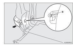
4. Remove the socket and bulb assembly (C) together by turning it anticlockwise and then remove the bulb by pulling it out.
