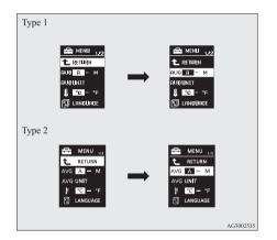
Press and hold the multi-information meter switch for about 2 seconds or more to switch in sequence from A (Auto reset mode) → M (Manual reset mode) → A (Auto reset mode). The setting is changed to the selected mode condition
