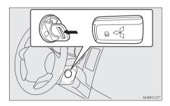
9. Turn the emergency key with keyless operation key to the "ON" position.
