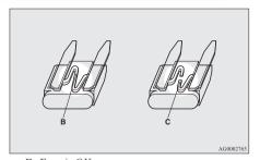
B- Fuse is OK C- Blown fuse
