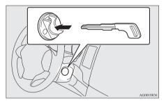
8. Insert the keyless operation key into the emergency key.
