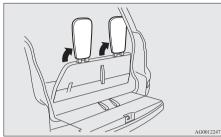
7. Lift up the whole of the third seat from the floor and fasten it to the front.
