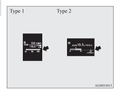
When the momentary fuel consumption surpasses the average fuel consumption, the momentary fuel consumption is displayed with a green bar graph. Be conscious of maintaining the momentary fuel consumption above the average fuel consumption, driving with the better fuel consumption can be possible. (Type 2)
