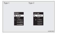
Press and hold the multi-information meter switch for about 2 seconds or more to change the setting to the selected unit.
