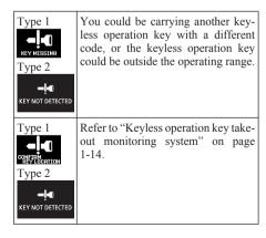
Even though you press a door or tailgate "LOCK" switch, the doors and tailgate will not lock.
