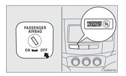
The front passenger's airbag is now deactivated and will not deploy until switched on again.
