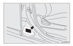
The label shows model code, engine model, transmission model and body colour code, etc. Please use this number when ordering replacement parts.
