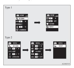
3. When you press and hold the multi-information meter switch for about 5 seconds or more, the buzzer sounds and all of the function settings are returned to the factory settings.
