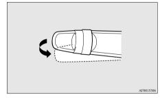
4. The headlamps will come on in the low beam setting for about 30 seconds. After the headlamps go off, the headlamps can be turned on again in the low beam setting for about 30 seconds by pulling the turn signal lever towards you within 60 seconds of turning the ignition switch to the "LOCK" position. To turn on the headlamps again after 60 seconds of turning the ignition switch to the "LOCK" position, repeat the process from step 1.
