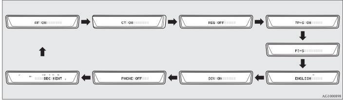
3. Press the TUNE switch (B) repeatedly to select the CT (Clock Time) mode.
