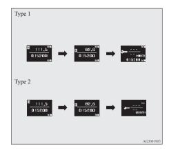
Press and hold the multi-information meter switch for about 2 seconds or more to display "-" and make it flash. (If there is no
