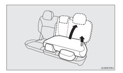
4. After returning the seatback, lightly push the seat and seatback to make sure they are set firmly in place.
