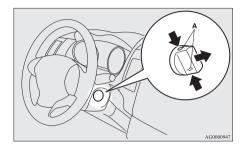
3. Insert the emergency key into the ignition switch, and turn while pushing.
