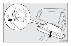
3. While pressing the side of the lower glove box, unhook the left and right hooks (B) and lower the lower glove box.
