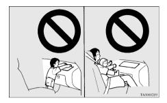
Use rearward facing child restraints in the rear seat or turn off the front passenger's airbag ON-OFF switch. (Refer to "To turn an airbag off" on page 2-34).
