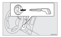
8. Insert the keyless operation key into the emergency key.
