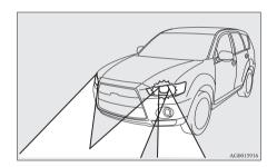
When the steering wheel is turned (on a curve, for example), the road ahead in the direction in which the car is being turned is illuminated. (The left bending lamp comes on when the car is turned leftward, and the right bending lamp comes on when the car is turned rightward.)
