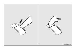
If the switch is fully pressed down/pulled up, the door window automatically opens/closes complete-ly.
