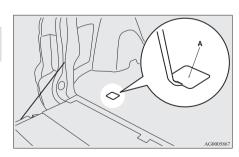
Insert the wheel nut wrench in the hole and lower the standard spare wheel by turning it anticlockwise.
