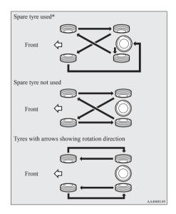
\*: If the spare tyre wheel differs from the standard tyre wheel, do not perform tyre rotation using a spare wheel.
