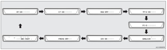
2. Press the TUNE switch (6) repeatedly to select the mode you wish to change. The order is:  $AF \rightarrow CT \rightarrow REG \rightarrow TP-S \rightarrow$ PI-S → Language of PTY display → SCV  $\rightarrow$  PHONE  $\rightarrow$  Function setup mode OFF.
