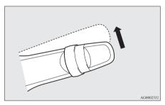
The wipers will operate once if the lever is moved to the "AUTO" position and the knob (C) is turned in the "+" direction when the ignition switch is in the "ON" position.
