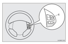
To increase your speed in small amounts, press the "ACC RES" switch for less than about 1 second and release it.
