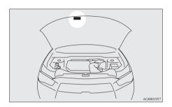
The plate shows the model code, engine model, transmission model and body colour code, etc. Please use this number when ordering replacement parts.
