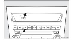
Automatic mode and manual mode is available for digital clock adjustment.
