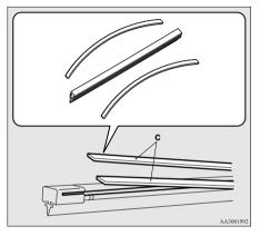
4. Insert the wiper blade into the arm, starting with the opposite end of the blade from the stopper. Make sure the hook (B) is fitted correctly in the grooves in the blade.
