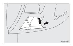
2. To put back the personal box, line up the personal box hook (C) with the clamp (D) on the instrument panel and push the box back in.
