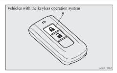
By locking the vehicle using the keyless entry system or the keyless operation system, the system preparation mode is activated. The buzzer makes an intermittent beeping sound and the security indicator (B) in the audio panel flashes for confirmation.
