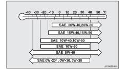
Select engine oil of the proper SAE viscosity number according to the atmospheric temperature.
