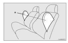
The label shown here is attached to the seatbacks with a side airbag.
