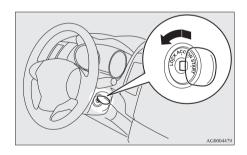
For vehicles equipped with an A/T, CVT or Twin Clutch SST, when removing the key, first set the selector lever (A/T or CVT) or gearshift lever (Twin Clutch SST) to the "P" (PARK) position, and then turn the key to the "LOCK" position, and remove it.
