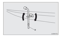
4. Always attach the tow rope to the towing hook. Otherwise, the instructions are the same as for "When being towed by another vehicle". 5. When finished towing, remove the towing hook, and stow it in the specified location. Refer to "Tools and jack" on page 6-08. When installing the bumper lid, align the
