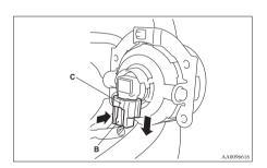
4. Turn the entire socket and bulb assembly (D) anticlockwise to remove it.
