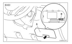
4. Referring to the fuse load capacity table, check the fuse pertaining to the problem.
