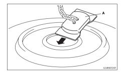
2. Turn the wheel nut wrench (B) clockwise to wind up the chain.
