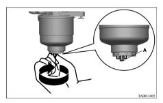
2. Operate the hand pump (B) slowly 6 or 7 times in order to force the water out through the drain plug (A).
