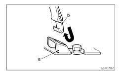
6. Push and pull the child restraint system in all directions to be sure it is firmly secured.
