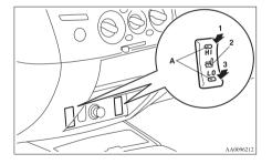
1 (HI)- Heater high (for quick heating).
