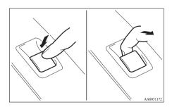
If the switch is fully pressed down/pulled up, the door window automatically opens/closes complete-ly.
