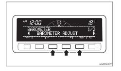
Adjust the barometer by pressing the function buttons.
