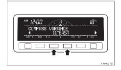
3. When the declination adjustment has been completed, press the "SET" function button.
