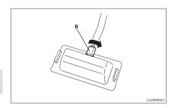
3. Remove the bulb by pulling out.
