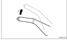
Firmly depress and hold the brake pedal, then pull the lever up without pushing the button at the end of hand grip.
