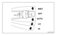
Keep the lever in the "OFF" position if the wind-screen is dirty and the weather is dry.
