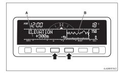
"+"- Adjustment of elevation
