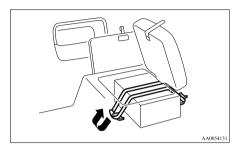
A band for securing a warning triangle is installed left under the rear seat.
