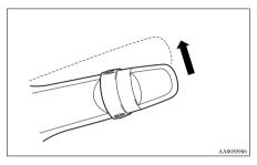
The wipers will operate once if the lever is moved to the "AUTO" position and the knob (A) is turned in the "+" direction when the ignition switch is "ON" position.
