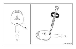
With the MITSUBISHI mark facing you, insert the cloth covered tip of a straight blade (or minus) screwdriver into the notch in the remote control switch case and use it to open the case.
