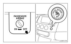
The front passenger's airbag OFF indication lamp will stay on to show that the front passenger's airbag is not operational. ("Front passenger's airbag OFF indication lamp" on page 2-31)
