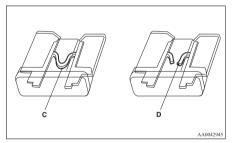
C- Fuse is OK D- Blown fuse
