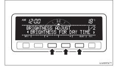
3. Use the function buttons to adjust the brightness.
