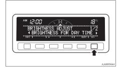
Press the "←" or "→" function button to select the setting you wish to adjust (daytime or nighttime). Then press the "SELECT" function button.
