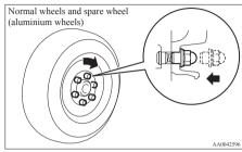
With a spare wheel, tighten the wheel nuts until the tapered parts of the wheel nuts make light contact with the seats of the wheel holes and the wheel is not loose.
