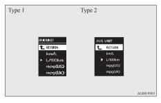
5. Press and hold the multi-information meter switch for about 2 seconds or more to change the setting to the selected unit.
