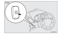
When the ignition switch is turned off, the status of the "AFS OFF" switch is held in memory.
