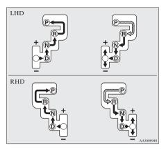
While depressing the brake pedal, move the selector lever through the gate.
