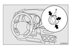
7. Insert the emergency key into the ignition switch.
