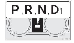
In addition, when the vehicle is driven with the gearshift lever in the "D" (DRIVE) position, the forward gear number is shown.
