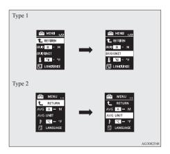
Press and hold the multi-information meter switch for about 2 seconds or more to display "AVG UNIT" (fuel consumption display unit setting).  4. Lightly press the multi-information meter switch to switch in sequence from km/L → L/100 km → mpg (US) → mpg (UK) → RE-TURN → km/I
