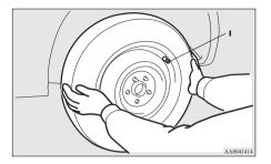
7. Finger-tighten the wheel nuts.
