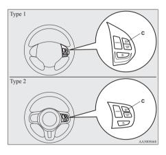
To increase your speed in small amounts, press the "ACC RES" switch for less than about 1 second and release it.
