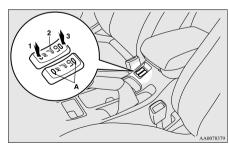
1 (HI)- Heater high (for quick heating).
