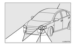
When the steering wheel is turned (on a curve, for example), the road ahead in the direction in which the car is being turned is illuminated. (The left bending lamp comes on when the car is turned leftward, and the right bending lamp comes on when the car is turned rightward.)
