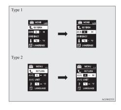
3. Press and hold the multi-information meter switch for about 2 seconds or more to switch in sequence from A (Auto reset mode) → M (Manual reset mode) → A (Auto reset mode). The setting is changed to the selected mode condition.
