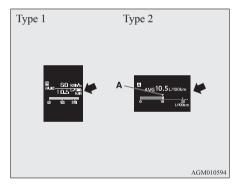
The "T" mark (A) in the momentary fuel gauge shows the average fuel consumption. (Type 2)
