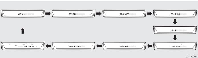
3. Press the TUNE switch (B) repeatedly to select the CT (Clock Time) mode. The order is: AF  $\rightarrow$  CT  $\rightarrow$  REG  $\rightarrow$  TP-S  $\rightarrow$  $PI-S \rightarrow Language of PTY display \rightarrow SCV$  $\rightarrow$  PHONE  $\rightarrow$  Function setup mode OFF. (Refer to "Function setup mode" on pages 5-25, 5-39.)
