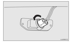
3. Remove the bulb by pulling it out.
