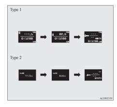
Press and hold the multi-information meter switch for about 2 seconds or more to display "> " and make it flash. (If there is no operation for about 10 seconds with flashing, the display returns to the previous screen.)  Lightly press the multi-information meter switch while the icon is flashing to change the display from "---" to "CLEAR". After this, the time until the next periodic inspection will be displayed.
