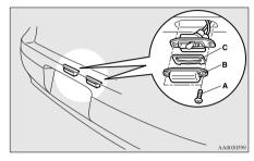
2. Remove the socket and bulb assemblies by turning it anticlockwise.
