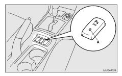
To return the system to the operating state, push the "SONAR" switch again. When the system returns to the operating state, the buzzer sounds once and the indication lamp illuminates.
