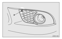
2. Pull the cover out in the direction of the arrow shown in the illustration.
