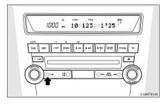
Push the CD button (2) if the discs are already in the CD autochanger.
