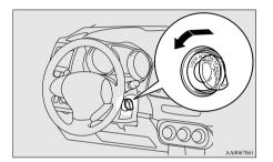
For vehicles with an A/T. CVT or Twin Clutch SST, when removing the key, first set the selector lever (A/T or CVT) or gearshift lever (Twin Clutch SST) to the "P" (PARK) position, and then turn the key to the "LOCK" position and remove it.
