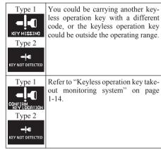
Even though you press the driver's or front passenger's door lock/unlock switch, the doors are not locked
