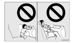
Use rearward facing child restraints in the rear seat or turn off the front passenger's airbag ON-OFF switch (if so equipped). (Refer to "To turn an airbag off" on page 2-23.)
