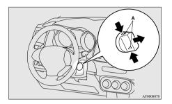
Insert the emergency key into the ignition switch.
