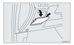
2. On vehicles with bottom cover, use the puller to loosen the 2 clips (A) and push down the bottom cover. The puller is in the fuse box in the engine compartment. Refer to "Fuse replacement" on page 8-25.
