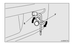
4. Always attach the tow rope to the towing hook. Otherwise, the instructions are the same as for "When being towed by another vehicle". 5. When finished towing, remove the towing hook, and stow it in the specified location. Refer to "Tools, jack and tyre repair kit" on page 6-06.
