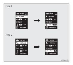
Press and hold the multi-information meter switch for about 2 seconds or more to switch in sequence from °C → °F → °C.
