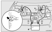
7. Connect one end of the other jumper cable to the negative (-) terminal of the booster battery, and the other end to the engine block of the vehicle with the discharged battery at the point farthest from the battery.
