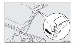
2. Remove the socket and bulb assembly by turning it anticlockwise.
