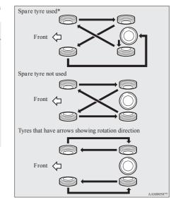
\*- If the spare tyre wheel differs from the standard tyre wheel, do not perform tyre rotation using a spare wheel.
