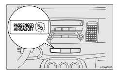
The indication lamp normally comes on when the ignition switch is turned to the "ON" position, and goes off a few seconds later.
