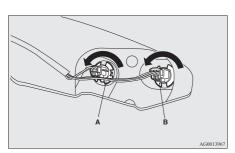
A- Rear turn-signal lamp B- Stop and tail lamp 3. Remove the bulb by pulling it out.
