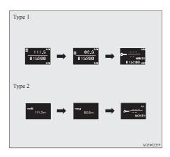
2. Press and hold the multi-information meter switch for about 2 seconds or more to display "> " and make it flash. (If there is no operation for about 10 seconds with flashing, the display returns to the previous screen.)
