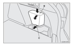
3. Check to make certain that the AWC control fluid level is always between the "MAX" and "MIN" level markings on the fluid reservoir and top up the fluid, if necessary.
