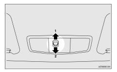
1 (DOOR) - The lamp illuminates when a door or the rear hatch is opened. It goes off about 15 seconds after the door or rear hatch is closed. However, the lamp goes off immediately in the following cases:
