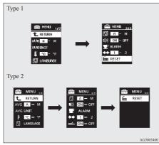
When you press and hold the multi-information meter switch for about 5 seconds or more, the buzzer sounds and all of the function settings are returned to the factory settings.
