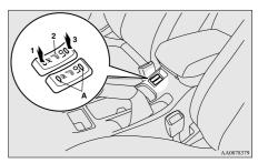
1 (HI)- Heater high (for quick heating).
