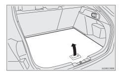
2. Pull the board forward until the front part is lowered.
