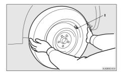
7. Finger-tighten the wheel nuts.
