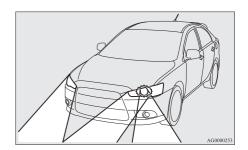
When the steering wheel is turned (on a curve, for example), the road ahead in the direction in which the vehicle is being turned is illuminated. (The left bending lamp comes on when the vehicle is turned leftward, and the right bending lamp comes on when the car is turned rightward.)
