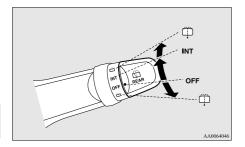
INT- The wiper operates continuously for several seconds then operates intermittently at intervals of about every 8 seconds
