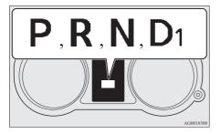
In addition, when the vehicle is driven with the gearshift lever in the "D" (DRIVE) position, the forward gear number is shown.
