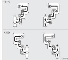
While depressing the brake pedal, move the selector lever through the gate.
