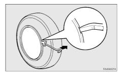
2. With the cover raised a little, pry it off completely using the jack bar. Insert the jack bar under the cover, and move it around the circumference, prying the cover away from the wheel little by little as you move the bar around.
