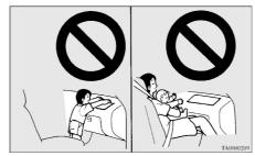
Use rearward facing child restraints in the rear seat or turn off the front passenger's airbag ON-OFF switch (if so equipped). (Refer to "To turn an airbag off" on page 2-25.)
