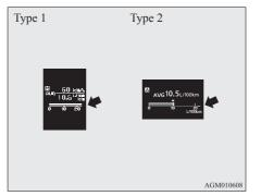
When the momentary fuel consumption surpasses the average fuel consumption, the momentary fuel consumption is displayed with a green bar graph. (Type 2)
