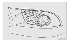
2. Pull the cover out in the direction of the arrow shown in the illustration.
