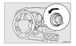
For vehicles with CVT or Twin Clutch SST, when removing the key, first set the selector lever (CVT) or gearshift lever (Twin Clutch SST) to the "P" (PARK) position, and then turn the key to the "LOCK" position and remove it.
