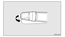
4. The headlamps will come on in the low-beam setting for about 30 seconds. After the headlamps go off, the headlamps can be turned on again in the low beam setting for about 30 seconds by pulling the turn signal lever towards you within 60 seconds of turning the ignition switch to the "LOCK" position. To turn on the headlamps again after 60 seconds of turning the ignition switch to the "LOCK" position, repeat the process from step 1.
