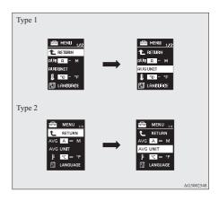
Press and hold the multi-information meter switch for about 2 seconds or more to display "AVG UNIT" (fuel consumption display unit setting).  4. Lightly press the multi-information meter switch to switch in sequence from km/L → L/100 km → mpg (US) → mpg (UK) → RE-TURN → km/L.
