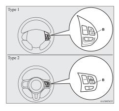
To slow down your speed in small amounts, press the "COAST SET" switch for less than about 1 second and release it.
