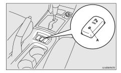
To return the system to the operating state, push the "SONAR" switch again. When the system returns to the operating state, the buzzer sounds once and the indication lamp illuminates.
