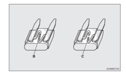
B- Fuse is OK C- Blown fuse
