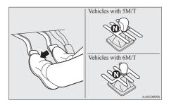
2. Release the clutch pedal. The "ASAG" display/indicator will turn on and the engine will stop automatically.
