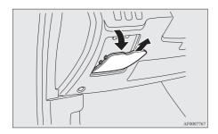
2. On vehicles with bottom cover, use the puller to loosen the 2 clips (A) and push down the bottom cover. The puller is in the fuse box in the engine compartment. Refer to "Fuse replacement" on page 8-27.
