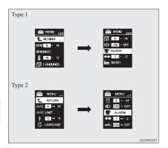
Press and hold the multi-information meter switch for about 2 seconds or more to display "ALARM" (rest time setting).
