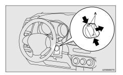
3. Insert the emergency key into the ignition switch and turn slowly while pushing.
