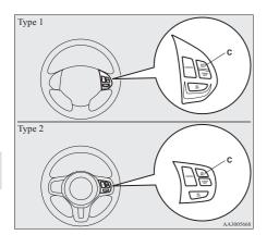
To increase your speed in small amounts, press the "ACC RES" switch for less than about 1 second and release it.
