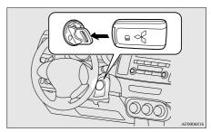
Turn the emergency key with keyless operation key to the "ON" position. The diesel preheat indication lamp will first illuminate, and then after a short time go out, indicating that preheating is completed.
