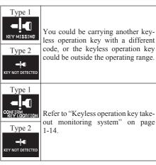
Even though you press the driver's or front passenger's door lock/unlock switch, or the rear hatch LOCK switch, the doors and rear hatch are not locked.
