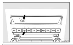
Automatic mode and manual mode are available for digital clock adjustment.
