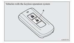
The settings mode can be toggled by pressing the UNLOCK switch. The mode can be confirmed from the number of times the buzzer sounds.
