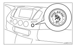
When the front passenger's airbag ON-OFF switch is turned OFF, the indication lamp will stay on to show that the front passenger's airbag is not operational.
