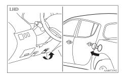
Open the fuel tank filler tube by slowly turning the cap anticlockwise.
