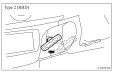
A- Parking brake lever stroke Type 1 8 to 9 notches Type 2 11 to 13 notches (Parking brake adjustment when pulled with the force of 200 N)
