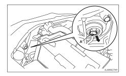
2. Remove the sealing cover (B).
