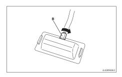
3. Remove the bulb by pulling out.
