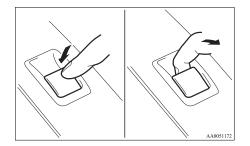
If the switch is fully pressed down/pulled up, the door window automatically opens/closes complete-ly.
