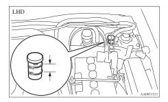
A rapid fluid loss indicates a leak in the clutch system which should be inspected by a MITSUBISHI MOTORS Authorized Service Point or another specialist and repaired immediately.
