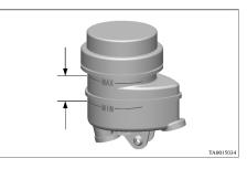
The brake fluid level is monitored by a float. When the brake fluid level falls below the "MIN" mark, the brake fluid warning lamp lights up.
