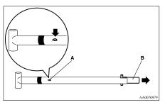
2. Reverse the inner handle (B) then, while pressing the snap pin (C), insert it into the outer handle (D) until it is locked by snap pin as illustrated.
