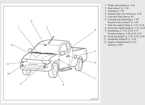
1. Wiper and washers p. 3-36 2. Rain sensor\* p. 3-36 3. Antenna p. 5-50 4. Outside rear-view mirrors p. 4-10 5. Fuel tank filler door p. 02 6. Locking and unlocking p. 1-02 Keyless entry system\* p. 1-04 7. Side turn-signal lamps p. 3-33, 8-24, 8-28 8. Front turn-signal lamps p. 3-33, 8-24, 8-27 9. Headlamps p. 3-30, 8-24, 3-31 Position lamps p. 3-30, 8-24, 8-27
