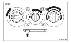
Warm air flows to the leg area and unheated or slightly warm air (depending upon temperature setting) flows to the upper part of the passenger compartment.
