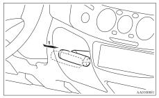
1- Firmly depress and hold the brake pedal, then pull the lever out.
