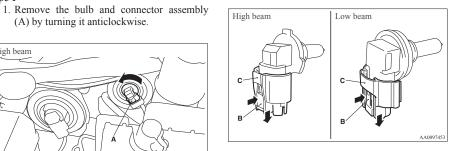
3. To install the bulb, perform the removal steps in reverse.
