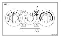
Push the switch again and the air conditioning compressor will stop and the indication lamp goes off.
