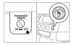
The front passenger's airbag OFF indication lamp will stay on to show that the front passenger's airbag is not operational. ("Front passenger's airbag OFF indication lamp" on page 2-31)
