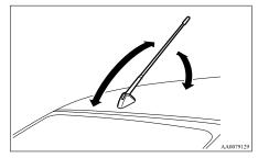
*To remove* Turn the pole (A) anticlockwise.
