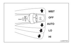
Keep the lever in the "OFF" position if the windscreen is dirty and the weather is dry. Wiper operation under these conditions can scratch the windscreen and damage the wipers.
