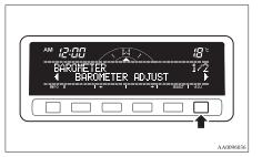
Press the "←" or "→" function button to select the "BAROMETER ADJUST" display. Then press the "SELECT" function button.
