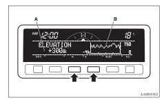
"+"- Adjustment of elevation The elevation increases by 100 m (400 ft) every time you lightly push the "+" button.
