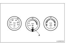
Push the switch again, and the air conditioning compressor will stop and the indication lamp goes off.
