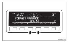
3. When the declination adjustment has been completed, press the "SET" function button.
