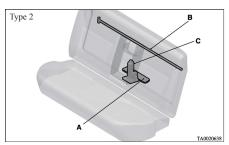
A- Tools B- Jack handle C- Jack Vehicles with rear retractable power window
