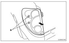
4. Remove each socket and bulb assembly by turning it anticlockwise.
