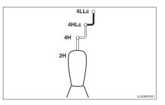
The transfer shift lever should be positioned in accordance with the following operating conditions: : Not push down the transfer shift lever : Push down the transfer shift lever
