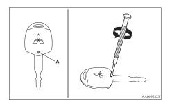
3. With the MITSUBISHI mark facing you, insert the cloth-covered tip of a straight blade (or minus) screwdriver into the notch in the remote control switch case and use it to open the case.
