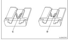
C- Fuse is OK D- Blown fuse
