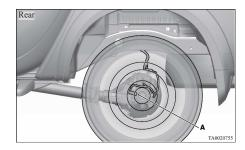
• The ABS becomes operative after the vehicle has accelerated to a speed in excess of approximately 10 km/h (6 mph). It stops operating when the vehicle decelerates to a speed below approximately 7 km/h (4 mph).
