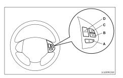
A- "ON OFF" switch Used to turn on and off the cruise control.
