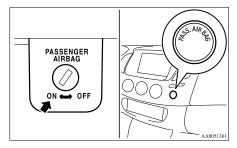
The front passenger's airbag OFF indication lamp goes off to show that the front passenger's airbag is operational.
