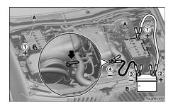
Connect one end of the other jumper cable to the negative (-) terminal of the booster battery (B), and the other end to the engine block of the vehicle with the discharged battery at the point farthest from the battery.
