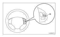
To slow down your speed in small amounts, press the "COAST SET" switch for less than about 1 second and release it.
