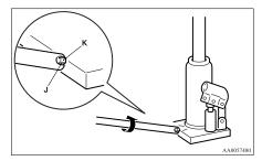
Press the piston down all the way, and turn the release valve clockwise as far as possible.
