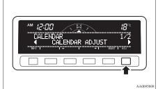
Press the "←" or "→" function button to select "CALENDAR ADJUST". Then press the "SELECT" function button.
