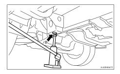
D- Front jacking point (2WD vehicles 16 inch wheels and 4WD vehicles)
