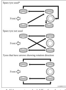
\*- If the spare tyre wheel differs from the standard tyre wheel, do not perform tyre rotation using a spare wheel.
