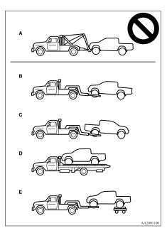
Towing the vehicle by a tow truck
