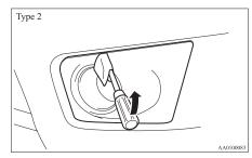
2. Turn the 3 bolts (A) anticlockwise to remove them. And then remove the lamp assembly.
