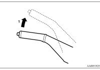
1- Firmly depress and hold the brake pedal, then pull the lever up without pushing the button at the end of hand grip.
