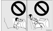
Use rearward facing child restraints in the rear seat or turn off the front passenger's airbag ON-OFF switch. (Refer to "To turn an airbag off" on page 2-22.)
