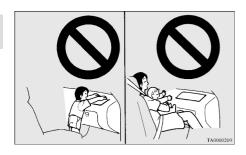
Use rearward facing child restraints in the rear seat or turn off the front passenger's airbag ON-OFF switch. (Refer to "To turn an airbag off" on page 3-23)
