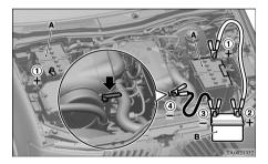
5. Connect one end of the other jumper cable to the negative (-) terminal of the booster battery (B), and the other end to the engine block of the vehicle with the discharged battery at the point farthest from the battery.
