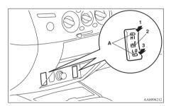
1 (HI)- Heater high (for quick heating).
