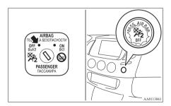
The front passenger's airbag OFF indication lamp will stay on to show that the front passenger's airbag is not operational. ("Front passenger's airbag OFF indication lamp" on page 2-32)
