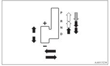
The lock button must be pushed while the brake pedal is depressed to move the selector lever
