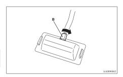
3. Remove the bulb by pulling out.
