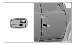
Set the inside lock knob (1) to the locked position, and close the door (2).
