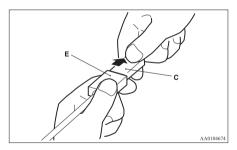
3. Fix the connector cable on the clips and close the glove box.
