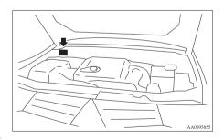
The plate shows model code and engine model, transmission model and body colour code, etc.
