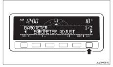
2. Press the "←" or "→" function button to select the "BAROMETER ADJUST" display. Then press the "SELECT" function button.
