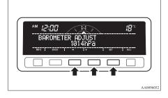
"+"- To adjust the barometer
