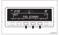
Press the "←" or "→" function button to select "km/L". Then press the "SET" function button. The display will flash twice, and the display unit will be updated to the selected one
