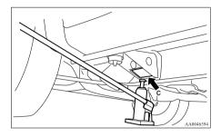
C- Front jacking point (2WD vehicles with 15 inch wheels)
