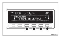
2. Press the "SET" function button. The display will flash twice and the barometer indication will return to the factory settings.
