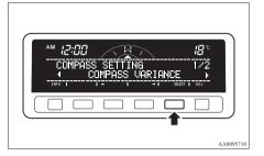
2. Press the function button for "←" or "→" to set the desired declination.
