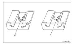
C- Fuse is OK D- Blown fuse
