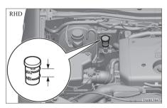
A rapid fluid loss indicates a leak in the clutch system which should be inspected by a MITSUBISHI MOTORS Authorized Service Point or another specialist and repaired immediately.
