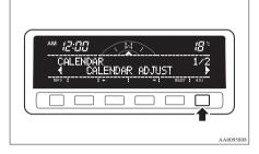
2. Press the "←" or "→" function button to select "CALENDAR ADJUST". Then press the "SELECT" function button.
