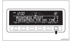
2. Press the "←" or "→" function button to select the setting you wish to adjust (daytime or nighttime). Then press the "SELECT" function button
