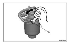
2. Pump the hand pump (B) until there are no more bubbles in the fuel coming out of the air plug (A). When doing this, place a cloth around the air plug (A) to prevent the escaping fuel from spraying out.
