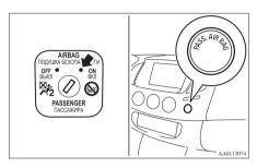
The front passenger's airbag OFF indication lamp goes off to show that the front passenger's airbag is operational.
