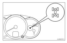
When the ignition switch is in the "ON" position, the 2WD/4WD operation indication lamp shows the shifting condition. The 2WD/4WD operation indication lamp illuminates at each transfer shift lever position as follows:
