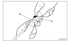
3. Fix the connector cable on the clips and close the glove box.
