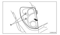
4. Remove each socket and bulb assembly by turning it anticlockwise.
