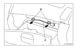
3. Connect the USB memory device (C) to the connector cable (A).
