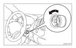
For vehicles with an A/T, when removing the key, first set the selector lever to the "P" (PARK) position, and then turn the key to the "LOCK" position, and remove it.
