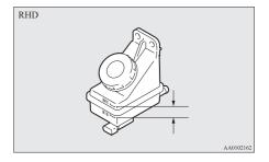
The brake fluid level is monitored by a float. When the brake fluid level falls below the "MIN" mark, the brake fluid warning lamp lights up. The fluid level falls slightly with wear of the brake pads, but this does not indicate any abnormality.
