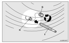
9. Remove the valve insert (J) by turning it anticlockwise using the valve remover (I). Put the removed valve insert in a clean place so it does not get dirty.
