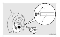
11. Holding the sealant bottle upside-down, squeeze it again and again to inject all of the sealant into the tyre.
