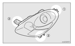
1. As shown in the illustration, insert the cut out area (A) on mounting bracket ① on to the bolt (B) remaining on the vehicle body, and latch the tab (C) on the fixture hole (D) to install the entire headlamp unit to the vehicle body.
