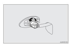
3. Pull the bulb out of the socket.
