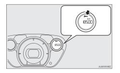
3. When the vehicle is inspected at a MITSUBISHI MOTORS Authorized Service Point, the driving distance or number of months remaining until the next inspection will be shown.
