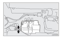
Before checking the auxiliary battery electrolyte level, remove the auxiliary battery's upper cover.
