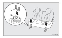
3. After installing the seat cushion, shake it lightly to check that it is properly fixed in position.
