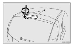
2. Turn the socket anticlockwise to remove it.
