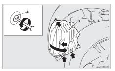
3. Turn the socket (C or D) anticlockwise to remove it.
