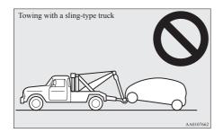
Towing with rear wheels raised off the ground
