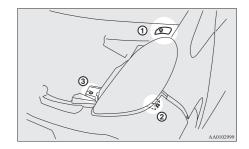
5. After pressing down on the bumper and fender joint from above to fit it in, fix it in place with the clip.
