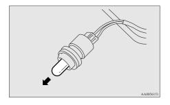
4. To install the bulb, perform the removal steps in reverse.
