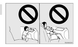
Use rearward facing child restraints in the rear seat or turn off the front passenger's airbag ON-OFF switch. (Refer to "To turn an airbag off" on page 3-23)
