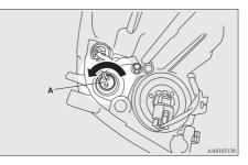
2. Pull the bulb out of the socket.
