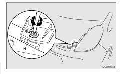
9. As shown in the illustration, shift the entire headlamp unit upward and then unlatch the tab (I) on the upper part of the headlamp to remove it from the vehicle.
