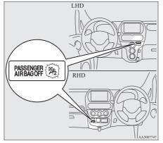
The indication lamp normally comes on when the electric motor switch is turned to the "ON" position, and goes off a few seconds later.
