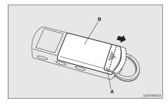
3. By moving the battery cover (B) in the direction indicated by the arrow, the tabs (C) on the battery cover will come out and the battery cover can be removed.
