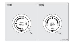
When the temperature control dial is set between the middle (•) and the "H" position The heating capability is the maximum.
