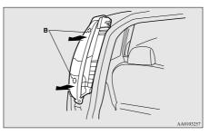
4. Turn the socket anticlockwise to remove it.
