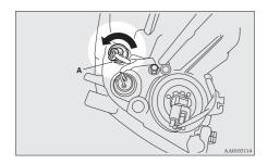
2. Pull the bulb out of the socket.
