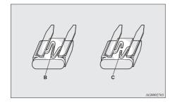
B- Fuse is OK C- Blown fuse
