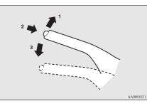
1- Firmly depress and hold the brake pedal, then pull the lever up slightly.
