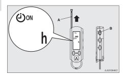
To turn the MiEV Remote off, press the power/communication switch (B) for 3 seconds or more and store the antenna (A).
