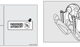
The front passenger's airbag is now deactivated and will not deploy until switched on again.
