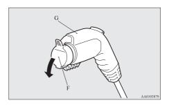
7. Connect the regular charge connector until a click sound is heard without pressing the button (H).
