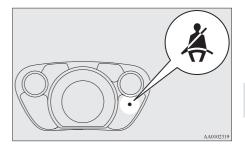
When the electric motor switch is turned to the "ON" position, if a driver or a front passenger has not fastened the seat belt, the warning lamp will illuminate.
