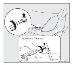
6. Slowly lift up the bumper and disconnect the joint between the bumper and fender.
