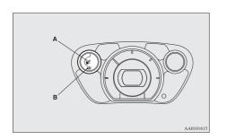
When the electric motor switch is in the "ON" position and the remaining bar of the energy level gauge shows 2 bars or less, the warning indicator (A) and the graduation (B) flash as follows:
