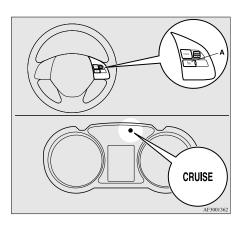
• If the cruise control is on when the following operation is performed, cruise control will be on automatically the next time you start the engine. The "CRUISE" indication lamp will also be on.
