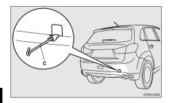
3. Use the wheel nut wrench (D) to firmly attach the towing hook.
