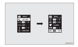
3. Press and hold the multi-information meter switch for about 2 seconds or more to switch in sequence from ON (with the green bar graph) → OFF (without the green bar graph) → ON (with the green bar graph).
