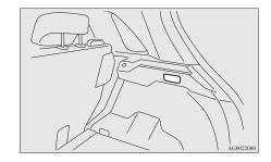
The lamp illuminates when the tailgate is opened, and goes out when the tailgate is closed
