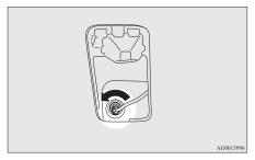
4. Remove the bulb by pulling it out.
