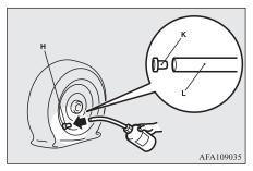
11. Holding the sealant bottle upside-down, squeeze it again and again to inject all of the sealant into the tyre.
