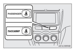
The lamp comes on when a person sits on the front passenger seat but does not fasten the seat belt. It goes off when the seat belt is subsequently fastened.
