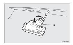
3. Remove the bulb by pulling it out.
