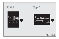
When the value of momentary fuel consumption surpasses the value of average fuel consumption, the momentary fuel consumption is displayed with a white bar graph. (Type 2)
