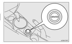
By pressing the drive mode-selector, the drive mode can be changed in order of "2WD", "4WD" AUTO and "4WD LOCK".
