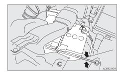
The electrolyte level must be between the specified limit on the outside of the battery. Replenish with distilled water as necessary. The inside of the battery is divided into several compartments; remove the cap from each compartment and fill to the upper mark. Do not top up beyond the upper mark because spillage during driving could cause damage. Check the electrolyte level at least once every 4 weeks, depending on the operating conditions.
