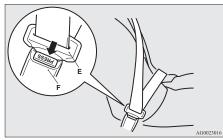
2. Push the button (G) on the buckle (C) using the latch plate (E) to disconnect the seat belt from the buckle.
