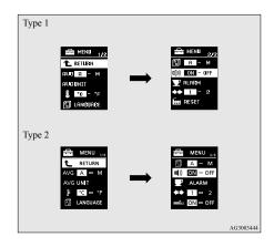
3. Press and hold the multi-information meter switch for about 2 seconds or more to switch in sequence from ON (operation sound on) → OFF (operation sound off) → ON (operation sound on). The setting is changed to the selected condition.
