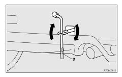
4. Always attach the tow rope to the towing hook. Otherwise, the instructions are the same as for "When being towed by another vehicle". When finished towing, remove the towing hook, and stow it in the specified location.
