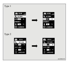
3. Press and hold the multi-information meter switch for about 2 seconds or more to switch in sequence from A or 1 (Auto reset mode) → M, 2 or P (Manual reset mode) → A or 1 (Auto reset mode).
