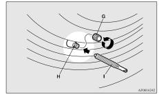
9. Remove the valve insert (J) by turning it anticlockwise using the valve remover (I). Put the removed valve insert in a clean place so it does not get dirty.
