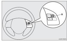
To slow down your speed in small amounts, push down the SET - switch for less than about 1 second and release it.
