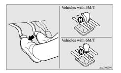
Release the clutch pedal. The "ssse" display/indicator will turn on and the engine will stop automatically.
