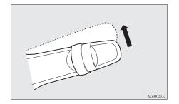
The wipers will operate once if the lever is moved to the "AUTO" position and the knob (C) is turned in the "+" direction when the ignition switch is in the "ON" position or the operation mode is in ON.
