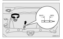
The engine oil used has a significant effect on the engine's performance, service life and startability. Be sure to use oil of the recommended quality and appropriate viscosity.
