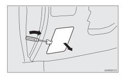
To put back the fuse lid, line up the fuse lid hook (A) with the clamp (B) on the instrument panel and push the lid back in.
