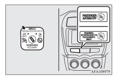
The front passenger's airbag is now deactivated and will not deploy until switched on again.
