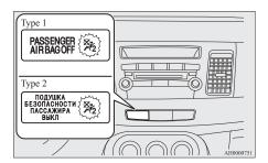
The indication lamp normally comes on when the ignition switch is turned to the "ON" position, and goes off a few seconds later.
