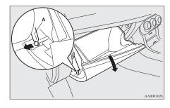
3. While pressing the side of the glove box, unhook the left and right hooks (B) and lower the glove box.
