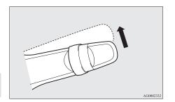
The wipers will operate once if the lever is moved to the "AUTO" position and the knob (C) is turned in the "+" direction when the ignition switch is in the "ON" position.
