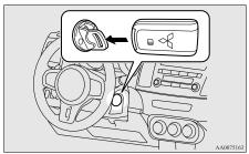
8. After turning the emergency key with the keyless operation key to the "ON" position, make sure that all warning lamps are functioning properly before starting the engine.
