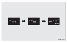
2. Press and hold the multi-information meter switch for about 2 seconds or more to display ">-" and make it flash. (If there is no operation for about 10 seconds with flashing, the display returns to the previous screen.)
