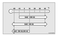
Select engine oil of the proper SAE viscosity number according to the atmospheric temperature.
