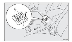
Heater high (for quick heating). 1 (HI)-
