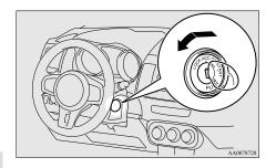
For vehicles with a Twin Clutch SST, when removing the key, first set the gearshift lever to the "P" (PARK) position, and then turn the key to the "LOCK" position and remove it.
