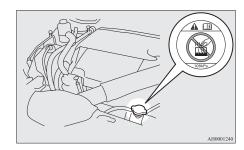
3. Confirm that the cooling fans are turning. If the fans (A) are not turning, stop the engine immediately and have it checked.
