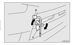
4. Secure the tow rope to the front towing hook.
