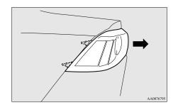
3. Remove the socket and bulb assemblies by turning them anticlockwise.
