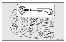
7. Insert the keyless operation key into the emergency key.
