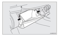
4. Remove the glove box fastener, and then remove the glove box.
