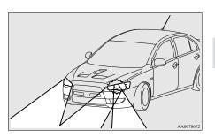
When the steering wheel is turned (on a curve, for example), the road ahead in the direction in which the vehicle is being turned is illuminated. (The left bending lamp comes on when the vehicle is turned leftward, and the right bending lamp comes on when the vehicle is turned rightward.)
