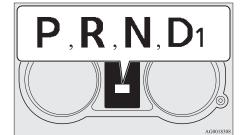
In addition, when the vehicle is driven with the gearshift lever in the "D" (DRIVE) position, the forward gear number is shown.
