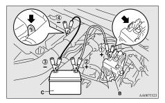
6. Connect one end of the other jumper cable to the negative (-) terminal of the booster battery, and the other end to the engine block of the vehicle with the discharged battery.
