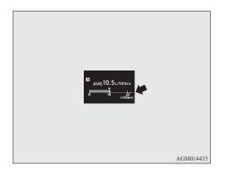
When the value of momentary fuel consumption surpasses the value of average fuel consumption, the momentary fuel consumption is displayed with a white bar graph.
