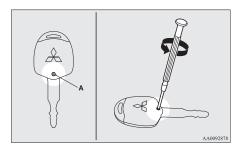
3. With the MITSUBISHI mark facing you, insert the clothcovered tip of a straight blade (or minus) screwdriver into the notch in the
