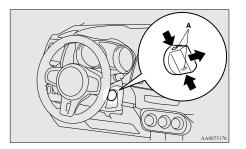
6. Insert the emergency key into the ignition switch.
