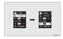
Press and hold the multi-information meter switch for about 2 seconds or more to switch in sequence from °C → °F → °C.
