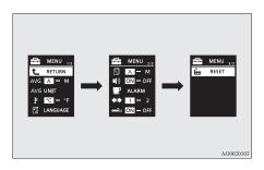
3. When you press and hold the multi-information meter switch for about 5 seconds or more, the buzzer sounds and all of the function settings are returned to the factory settings.
