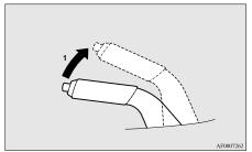
1- Firmly depress and hold the brake pedal. then pull the lever up without pushing the button at the end of hand grip.
