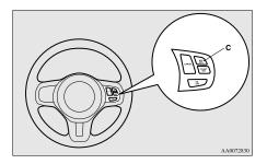
To increase your speed in small amounts, press the "ACC RES" switch for less than about 1 second and release it.
