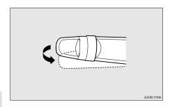
4. The headlamps will come on in the lowbeam setting for about 30 seconds. After the headlamps go off, the headlamps can be turned on again in the low beam setting for about 30 seconds by pulling the turn signal lever towards you within 60 seconds of turning the ignition switch to the "LOCK" position. To turn on the headlamps again after 60 seconds of turning the ignition switch to the "LOCK" position, repeat the process from step 1.
