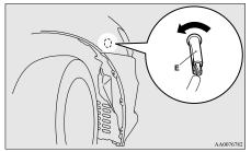
4. Pull the bulb out of the socket.
