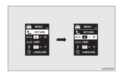
Press and hold the multi-information meter switch for about 2 seconds or more to switch in sequence from A or 1 (Auto reset mode) → M, 2 or P (Manual reset mode) → A or 1 (Auto reset mode).
