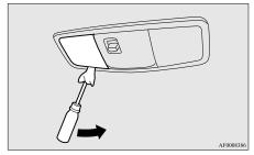
2. While holding down the tab (A), pull out the bulb.
