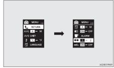
3 Press and hold the multi-information meter switch for about 2 seconds or more to switch in sequence from 1 (turn-signal sound 1)  $\rightarrow$ 2 (turn-signal sound 2)  $\rightarrow$  1 (turn-signal sound 1).
