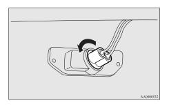
3. Remove the bulb by pulling it out.
