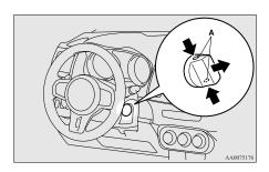
3. Insert the emergency key into the ignition switch and turn slowly while pushing.
