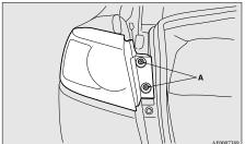
2. Remove the lamp unit in the rear direction.
