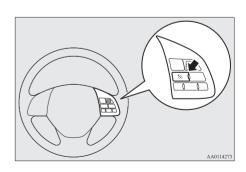
The set speed is cancelled when the ACC is turned off or the operation mode is set to "OFF".
