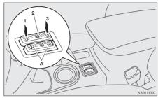
1 (HI) - Heater high (for quick heating).
