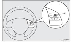
The set speed is increased each about 5 km/h (3 mph) per about 0.5 second.
