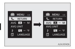
3. Press and hold the multi information display switch for about 2 seconds or more to switch from A/1 (Auto reset mode) to M/2/P (Manual reset mode), or from M/2/P to A/1.
