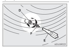
When removing and screwing in the valve insert using the valve remover, turn the valve remover by hand. Using a tool to turn the valve remover could damage it. 12. After injecting the sealant, securely fit the valve remover (E) into the end of the filler hose (J) to prevent sealant from leaking from the empty bottle.
