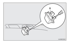
3. Remove the bulb from the socket.
