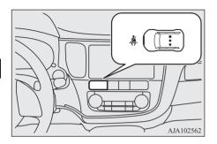
If the operation mode of the power switch is put in ON while a seat belt is not fastened, the warning lamp comes on for approximately 30 seconds to remind the rear passenger to fasten the seat belt.
