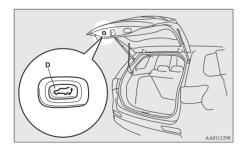
If the close switch on the inside of the electric tailgate is pressed, the electric tailgate closes after the warning buzzer sounds 3 times and the hazard warning flasher brinks 2 times.
