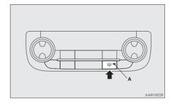
If you are carrying the keyless operation key, you can start the Plug-in Hybrid EV System.
