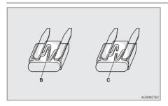
B- Fuse is OK C- Blown fuse
