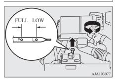
The engine oil used has a significant effect on the engine's performance, service life and startability. Be sure to use oil of the recommended quality and appropriate viscosity.
