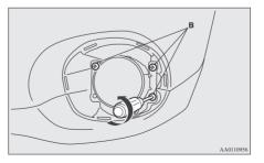
3. Turn the bulb or socket anticlockwise to remove it.
