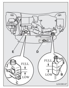
B: Reserve tank for engine cooling C: Reserve tank for EV cooling system Add coolant to the radiator and/or reserve tank if necessary. (Refer to the "Maintenance" section.)
