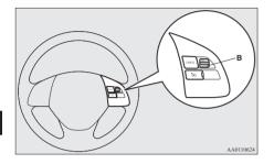
To slow down your speed in small amounts, push down the SET - switch (B) for less than about 1 second and release it.
