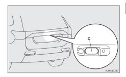
If the open switch is pressed with the tailgate and all doors are unlocked, the electric tailgate opens after the warning buzzer sounds 4 times and the hazard warning flasher brinks 2 times.
