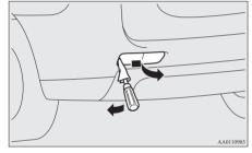
2. Turn the socket (A) anticlockwise to remove it, and then pull the bulb out of the socket.
