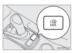
If the battery save mode is activated, the following image is displayed on the information screen in the multi-information display.
