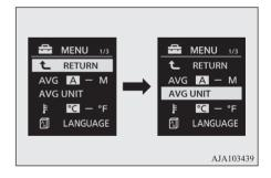
Press and hold the multi information display switch for about 2 seconds or more to display "AVG UNIT".
