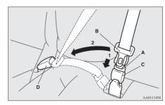
4. Pull the belt slightly to adjust slackness as desired
