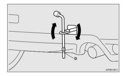
4. Always attach the tow rope to the towing
