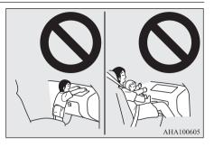
Use rearward facing child restraints in the rear seat or turn off the front passenger's airbag ON-OFF switch (if so equipped). (Refer to "To turn an airbag off" on page 4-28)
