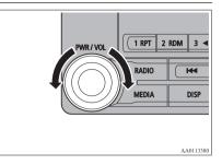
Turn the PWR/VOL key clockwise to increase, and counter- clockwise to decrease the volume.
