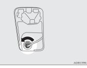
4. Remove the bulb by pulling it out.
