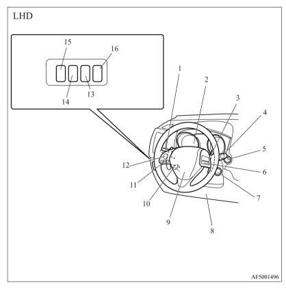
1. Combination headlamps and dipper switch p. 5-48 Turn-signal lever p. 5-55 Front fog lamp switch\* p. 5-56 Rear fog lamp switch p. 5-56 Headlamp washer switch\* p. 5-62 E00100108663
