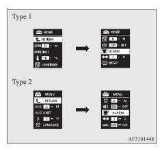
3. Press and hold the multi-information meter switch for about 2 seconds or more to display "ALARM" (rest time setting).
