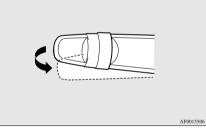
4. The headlamps will come on in the lowbeam setting for about 30 seconds. After the headlamps go off, the headlamps can be turned on again in the low beam setting for about 30 seconds by pulling the turn signal lever towards you within 60 seconds of turning the ignition switch to the "OFF" position or putting the operation mode in OFF.
