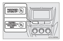
The indicator normally illuminates when the ignition switch is turned to the "ON" position or the operation mode is put in ON, and goes off a few seconds later.
