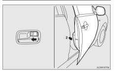
Set the inside lock knob (1) to the locked position, and close the door (2).
