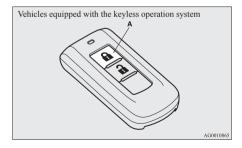
Driver's and front passenger's door lock/unlock switches\*
