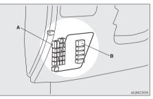
A- Main fuse block B- Sub fuse block 1. Insert a straight blade (or minus) screwdriver into the notch of the fuse lid and pry gently to remove it.
