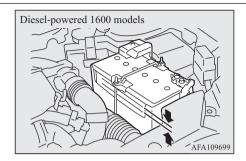
The electrolyte level must be between the specified limit on the outside of the battery. Replenish with distilled water as necessary. The inside of the battery is divided into several compartments; remove the cap from each compartment and fill to the upper mark. Do not top up beyond the upper mark because spillage during driving could cause damage.
