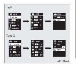
3. When you press and hold the multi-information meter switch for about 5 seconds or more, the buzzer sounds and all of the function settings are returned to the factory settings.
