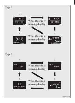
1- Odometer (Type 1)/Tripmeter **A** 2- Odometer (Type 1)/Tripmeter **B**
