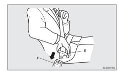
4. Make sure the lap belt is positioned as low as possible on the hips and pull the shoulder belt to adjust the slackness of the lap belt.
