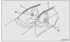
6- Side airbag modules\*7- Curtain airbag modules\*
