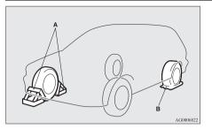
• Be sure to apply chocks or blocks to the correct tyre when jacking up the vehicle. If the vehicle moves while jacked up, the jack could slip out of position, leading to an accident.
