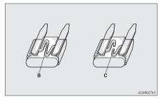
B- Fuse is OK C- Blown fuse
