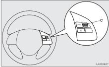
To increase your speed in small amounts, push up the RES + switch for less than about 1 second and release it.
