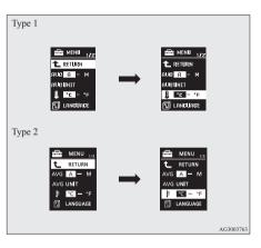
Press and hold the multi-information meter switch for about 2 seconds or more to switch in sequence from °C → °F → °C.
