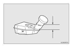
The fluid level is monitored by a float. When the fluid level falls below the "MIN" mark, the brake fluid warning lamp lights up. The fluid level falls slightly with wear of the brake pads, but this does not indicate any abnormality.
