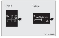
When the value of momentary fuel consumption surpasses the value of average fuel consumption, the momentary fuel consumption is displayed with a white bar graph. (Type 2) Be conscious of maintaining the value of momentary fuel consumption below the value of average fuel consumption, driving with the bet-ter fuel consumption can be possible.
