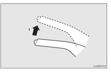
1- Firmly depress and hold the brake pedal, then pull the lever up without pushing the button at the end of hand grip.
