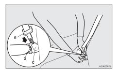
3. Retract the seat belt and remove it from the seat belt guide (A).
