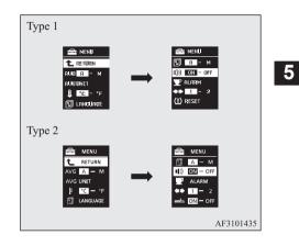
3. Press and hold the multi-information meter switch for about 2 seconds or more to switch in sequence from ON (operation sound on)  $\rightarrow$  OFF (operation sound off)  $\rightarrow$  ON (operation sound on). The setting is changed to the selected condition.
