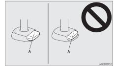
• The head restraints for the seats differ in shape and size. When installing head restraints, make sure the head restraints are fitted in their respective seats and do not install the head restraints in the wrong direction.
