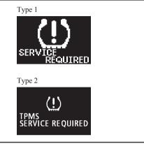
Each tyre, including the spare (if so equipped), should be checked monthly when cold and inflated to the inflation pressure recommended by the vehicle manufacturer on the tyre inflation pressure label. (If your vehicle has tyres of a different size than the size indicated on the tyre inflation pressure label, you should determine the proper tyre inflation pressure for those tyres.)
