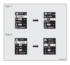
Press and hold the multi-information meter switch for about 2 seconds or more to switch in sequence from A or 1 (Auto reset mode) → M, 2 or P (Manual reset mode) → A or 1 (Auto reset mode).
