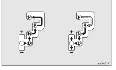
While depressing the brake pedal, move the selector lever through the gate. Move the selector lever through the gate.
