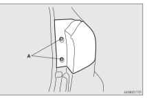
2. Turn the socket and bulb assembly anticlockwise to remove it.
