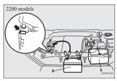
7. Connect one end of the other jumper cable to the negative (-) terminal of the booster battery, and the other end to the engine block of the vehicle with the discharged battery at the point farthest from the battery.
