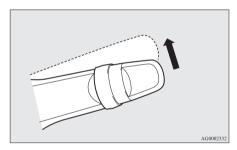
The wipers will operate once if the lever is moved to the "AUTO" position and the knob (C) is turned in the "+" direction when the ignition switch is in the "ON" position or the operation mode is in ON.
