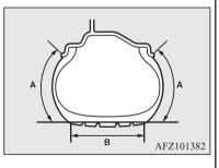
• The vehicle has been driven with the tyre almost completely flat.
