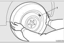
7. Turn the wheel nuts clockwise by hand to initially tighten them.
