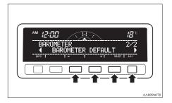
Press the "SET" function button. The display will flash twice and the barometer indication will return to the factory settings.
