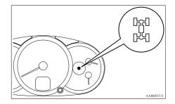
When the ignition switch is in the "ON" position, the 2WD/4WD operation indication lamp shows the shifting condition. The 2WD/4WD operation indication lamp illuminates at each transfer shift lever position as follows:
