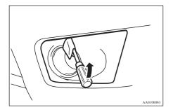
Turn the 3 bolts (A) anticlockwise to remove them. And then remove the lamp assembly.
