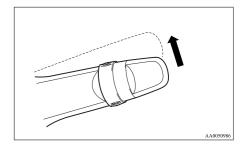
The wipers will operate once if the lever is moved to the "AUTO" position and the knob (A) is turned in the "+" direction when the ignition switch is "ON" position.
