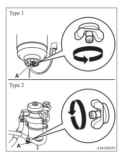
2. Operate the hand pump (B) slowly 6 or 7 times in order to force the water out through the drain plug (A).
