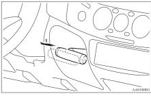
1- Firmly depress and hold the brake pedal, then pull the lever out.
