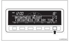
Press the "←" or "→" function button to select the setting you wish to adjust (daytime or nighttime). Then press the "SELECT" function button.
