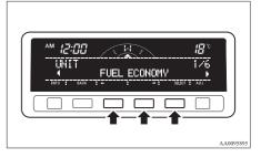
2. Press the "←" or "→" function button to select "km/L". Then press the "SET" function button. The display will flash twice, and the display unit will be updated to the selected one.
