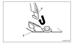
Push and pull the child restraint system in all directions to be sure it is firmly secured
