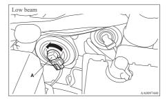
Depress the tab (B) on the harness connector and pull the harness connector (C) to remove it.
