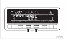
When the declination adjustment has been completed, press the "SET" function button
