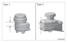
The brake fluid level is monitored by a float. When the brake fluid level falls below the "MIN" mark, the brake fluid warning lamp lights up.
