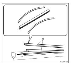
Insert the wiper blade into the arm, starting with the opposite end of the blade from the stopper. Make sure the hook
