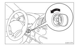
For vehicles with an A/T, when removing the key, first set the selector lever to the "P" (PARK) position, and then turn the key to the "LOCK" position, and remove it.
