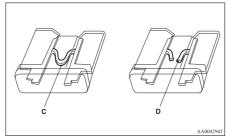
C- Fuse is OK D- Blown fuse
