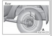
The ABS becomes operative after the vehicle has accelerated to a speed in excess of approximately 10 km/h (6 mph). It stops operating when the vehicle decelerates to a speed below approximately 7 km/h (4 mph).
