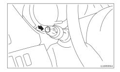
• If the ignition switch is in the "ON" or "ACC" position and the headlamps are on, the headlamp washer operates together with the windscreen washer the first time the windscreen washer lever is pulled.
