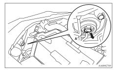
2. Remove the sealing cover (B).
