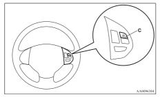
To increase your speed in small amounts, press the "ACC RES" switch for less than about 1 second and release it. Each time you press the "ACC RES" switch, your vehicle will go about 1.6 km/h (1 mph) faster.
