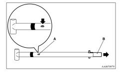
2. Reverse the inner handle (B) then, while pressing the snap pin (C), insert it into
