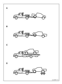
Be sure to shift the transfer shift lever to "2H" position and transport the vehicle with the driving wheels on a carriage (Type A, C or D) as illustrated.
