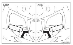
Firmly depress and hold the brake pedal, then pull the lever out slightly and turn it clockwise (LHD) or anticlockwise (RHD).
