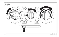
Warm air flows to the leg area and unheated or slightly warm air (depending upon temperature setting) flows to the upper part of the passenger compartment.
