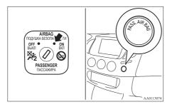
The front passenger's airbag OFF indication lamp goes off to show that the front passenger's airbag is operational.
