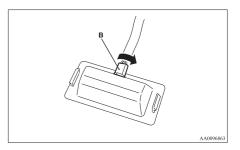
3. Remove the bulb by pulling out.
