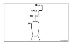
The transfer shift lever should be positioned in accordance with the following operating conditions:
