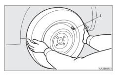
7. Temporarily tighten the wheel nuts by hand until the tapered parts of the wheel nuts make light contact with the seats of the wheel holes and the wheel is not loose.
