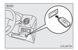
• Do not insert into the key slot anything other than the keyless operation key. This could
