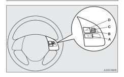
A- CRUISE CONTROL ON/OFF switch Used to turn on and off the cruise con-
