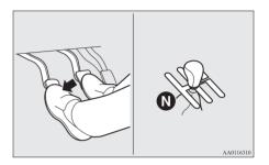
3. Release the clutch pedal. The engine will stop automatically.
