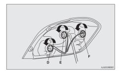
Bulb type stop and tail lamps
