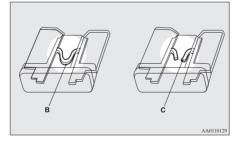
B- Fuse is OK C- Blown fuse
