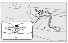
3. Fix the terminal part (A) of the connector cable on the clip and close the glove box.
