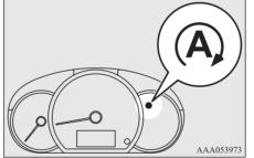
[For vehicles with M/T] 1. Stop the vehicle. 2. Depressing the brake pedal. The engine will stop automatically.
