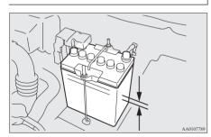
The electrolyte level must be between the specified limit on the outside of the battery. Replenish with distilled water as necessary. The inside of the battery is divided into several compartments; remove the cap from each compartment and fill to the upper mark. Do not top up beyond the upper mark because spillage during driving could cause damage. Check the electrolyte level at least once every 4 weeks, depending on the operating conditions.
