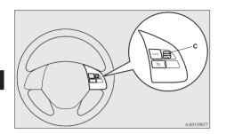
To increase your speed in small amounts, push up the RES + switch (C) for less than about 1 second and release it.
