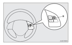
To slow down your speed in small amounts, push down the SET - switch (B) for less than about 1 second and release it.
