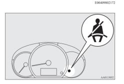
If the ignition switch is turned to the "ON" position or the operation mode is put in ON while a seat belt is not fastened, the warning lamp comes on and the tone sounds for about 6 seconds to remind the driver and the front passenger to fasten the seat belt.
