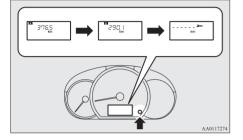
Press and hold the multi-information display switch for about 1 second or more to make the spanner mark start flashing. (If there is no operation for about 10 seconds with flashing, the display will revert to its original indication.)
