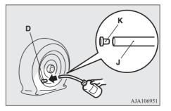
11. Holding the sealant bottle upside-down, squeeze it again and again to inject all of the sealant into the tyre.
