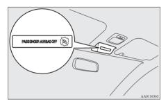
The indication lamp normally comes on when the ignition switch is turned to the "ON" position or the operation mode is put in ON, and goes off a few seconds later.
