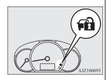
• If there is a fault in the steering wheel lock, the warning lamp illuminates and the inner buzzer sounds. Immediately stop the vehicle in a safe place and contact a MITSUBISHI MOTORS Authorized Service Point.
