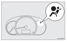
There is a Supplemental Restraint System ("SRS") warning lamp on the instrument panel. The system checks itself every time the ignition switch is turned to the "ON" position or the operation mode is put in ON. The SRS warning lamp will come on for several seconds and then go out.
