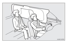
Deployment of side airbags and curtain airbags
