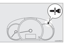
When the operation mode is in any mode other than OFF, if you close all the doors and the tailgate then try to lock the doors and tailgate by pressing the driver's door switch, or the tailgate switch, a warning lamp will blink and the outer buzzer will sounds for approximately 3 seconds and you cannot lock the doors and tailgate.
