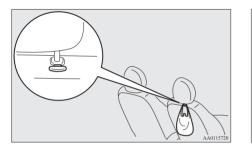
The grip is to support the body by hand while seated in the vehicle.
