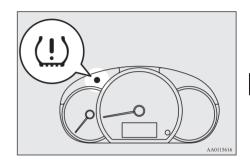
When the ignition switch is turned to the "ON" position or the operation mode is put in ON, the tyre pressure monitoring system warning lamp normally illuminates and goes off a few seconds later.
