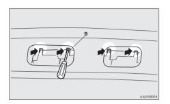
4. Gently close the tailgate, remove the lamp unit, and turn the socket anticlock-wise to remove it.
