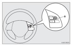
• When you release the SET - switch (B), the vehicle speed will be set.
