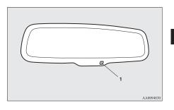
When the ignition switch is turned to the "ON" position or the operation mode is put in ON, the reflection factor of the mirror is automatically changed.
