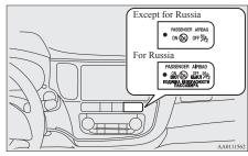
The both indicator normally comes on when the ignition switch is turned to the "ON" position or the operation mode is put in ON, and goes off a few seconds later.
