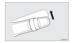
The wipers will operate once if the lever is moved to the "AUTO" position and the knob (C) is turned in the "+" direction when the ignition switch is in the "ON" position or the operation mode is in ON.
