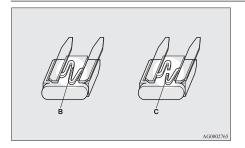
B- Fuse is OK C- Blown fuse
