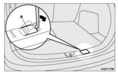
2. Loosen the tyre hanger installation bolt by turning it anticlockwise with the wheel nut wrench
