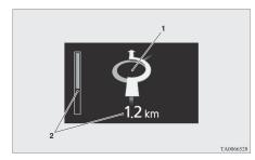
1- Guidance display Shows the direction of vehicle travel and the guidance location.
