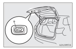
If the close switch on the inside of the electric tailgate is pressed, the electric tailgate closes after the warning buzzer sounds.
