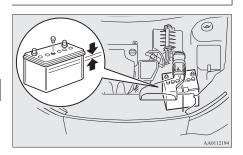
The electrolyte level must be between the specified limit on the outside of the battery. Replenish with distilled water as necessary. The inside of the battery is divided into several compartments; remove the cap from each compartment and fill to the upper mark. Do not top up beyond the upper mark because spillage during driving could cause damage. Check the electrolyte level at least once every 4 weeks, depending on the operating condi-
