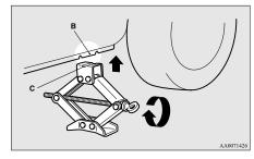
4. Insert the jack bar (D) into the wheel nut wrench (E). Then put the end of the jack bar into the shaft's jack end, as shown in the illustration
