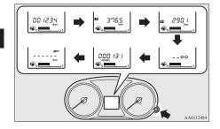
Press and hold the multi information display switch for about 2 seconds or more to make the spanner mark start flashing.
