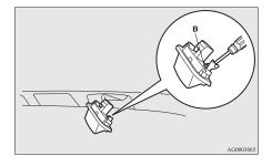
3. Remove the bulb from the socket.
