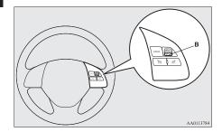
If the current vehicle speed is lower than about 30 km/h (19 mph) (settable minimum speed), the set speed is set at about 30 km/h (19 mph).
