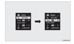
3. Press and hold the multi information display switch for about 2 seconds or more to switch from A/1 (Auto reset mode) to M/2/P (Manual reset mode), or from M/2/P to A/1.
