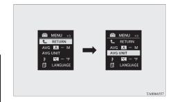
3. Press and hold the multi-information meter switch for about 2 seconds or more to display "AVG UNIT" (fuel consumption display unit setting).
