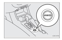
If you press the switch, you can change the drive mode in the order of 4WD ECO, 4WD AUTO, 4WD LOCK, 4WD ECO.
