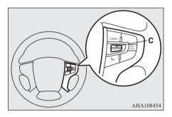
To increase your speed in small amounts, push up the RES + switch (C) for less than about 1 second and release it.
