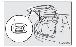
If the close switch on the inside of the electric tailgate is pressed, the electric tailgate closes after the warning buzzer sounds and the hazard warning flasher blinks.
