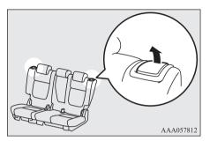
To adjust the seatback, pull the lever up and adjust the seatback by hand to the desired position, and release the lever.
