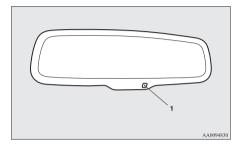
When the ignition switch is turned to the "ON" position, the reflection factor of the mirror is automatically changed.
