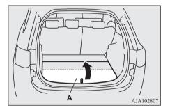
To use the luggage floor box in the rear seat side, insert your hand in the gap (B) and raise the board (A) to the seat side.
