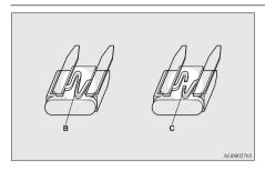
B- Fuse is OK C- Blown fuse
