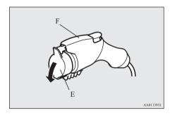
7. Connect the normal charge connector until a click sound is heard without pressing the button (G).
