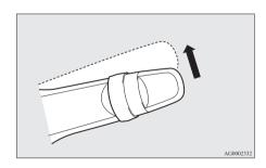
The wipers will operate once if the lever is moved to the "AUTO" position and the knob (C) is turned in the "+" direction when the operation mode is in ON.
