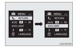
3. Press and hold the multi information display switch for about 2 seconds or more to display "AVG UNIT".
