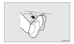
Put on an accelerator pedal to the pedal stroke end. (over a detent that makes pedal reaction force bigger before pedal stroke end)
