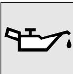
This lamp illuminates when the ignition switch is turned to the “ON” position, and goes off after the engine has started. If it illuminates while the engine is running,
