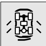
This lamp illuminates when a door or the backdoor is either open or incompletely closed.
