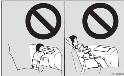
Use rearward facing child restraints in the rear seat or turn off the front passenger’s airbag ON-OFF switch. (Refer to “To turn an airbag off” on page 4-40.)
