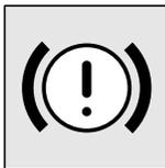
This lamp illuminates when the ignition switch is turned to the “ON” position, and goes off after a few seconds. Always make sure that the lamp goes off before driving.
