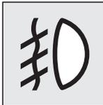
This indication lamp illuminates while the front fog lamps are on.
