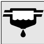
This indication lamp illuminates when the ignition switch is turned to the “ON” position and goes off after the engine has started. If it lights up while the engine is
