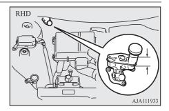
The fluid level is monitored by a float. When the fluid level falls below the "MIN" mark, the brake fluid warning lamp lights up.
