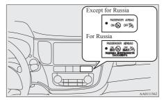
The both indicator normally comes on when the operation mode of the power switch is put in ON, and goes off a few seconds later.
