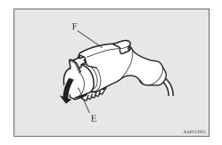
7. Connect the normal charge connector until a click sound is heard without pressing the release button (G).
