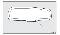
When the operation mode of the power switch is put in ON, the reflection factor of the mirror is automatically changed.
