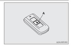
The settings mode can be toggled by pressing the UNLOCK switch. The mode can be confirmed from the number of times the buzzer sounds.
