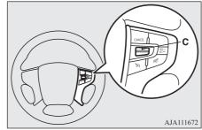
The set speed is increased each about 5 km/h (3 mph) per about 0.5 second.
