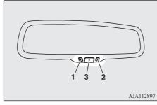
When the operation mode of the power switch is put in ON, the green indicator (1) illuminates and the reflection factor of the mirror is automatically changed.
