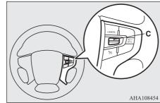
To increase your speed in small amounts, push up the RES + switch (C) for less than about 1 second and release it.
