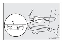
If the open switch is pressed with the tailgate and all doors are unlocked, the electric tailgate opens after the warning buzzer sounds and the hazard warning flasher blinks.
