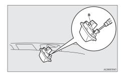
3. Remove the bulb from the socket.
