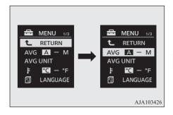
3. Press and hold the multi information display switch for about 2 seconds or more to switch from A/1 (Auto reset mode) to M/2/P (Manual reset mode), or from M/2/P to A/1
