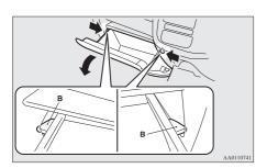
4. Remove the glove box fastener (C), and then remove the glove box.
