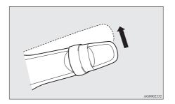
The wipers will operate once if the lever is moved to the "AUTO" position and the knob (C) is turned in the "+" direction when the ignition switch is in the "ON" position.
