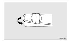
4. The headlamps will come on in the low beam setting for about 30 seconds. After the headlamps go off, the headlamps can be turned on again in the low beam setting for about 30 seconds by pulling the turn signal lever towards you within 60 seconds of putting the operation mode in OFF.
