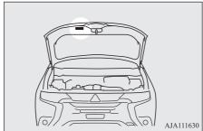
The plate shows the model code, engine model, transaxle model and body colour code, etc.
