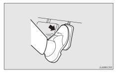
Put on an accelerator pedal to the pedal stroke end. (over a detent that makes pedal reaction force bigger before pedal stroke end)
