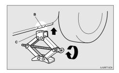
Check that the flange portion at the jacking point fits in the groove at the top of the jack.
