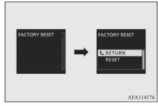
Press the ➤ switch or ➤ switch to select "RESET", and then press and hold the © switch for approximately 5 seconds or more to confirm the setting.
