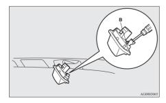
3. Remove the bulb from the socket.
