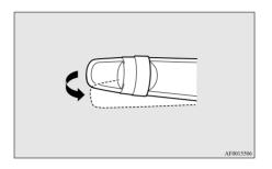
4. The headlamps will come on in the low beam setting for approximately 30 seconds. After the headlamps go off, the headlamps can be turned on again in the low beam setting for approximately 30 seconds by pulling the turn signal lever towards you within 60 seconds of turning the ignition switch to the "LOCK" position or putting the operation mode in OFF.
