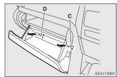
4. Pull the glove box from the bottom to remove it.
