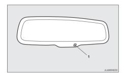
When the ignition switch is turned to the "ON" position or the operation mode is put in ON, the reflection factor of the mirror is automatically changed.
