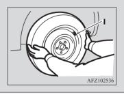
7. Turn the wheel nuts clockwise by hand to initially tighten them.
