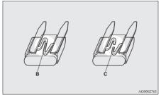
B- Fuse is OK C- Blown fuse
