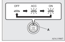
OFF- The indication lamp (A) on the engine switch turns off.
