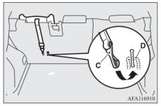
6. Push and pull the child restraint system in all directions to be sure it is secured.
