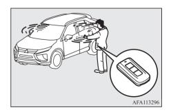
• If the keyless operation key battery is wearing out or there are strong electromagnetic waves or noise present, the operating range may become smaller and operation may become unstable
