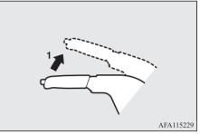
1- Firmly depress and hold the brake pedal, then pull the lever up without pressing the button at the end of hand grip.
