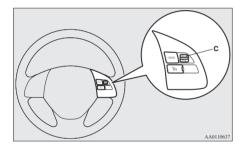
To increase your speed in small amounts, push up the "RES +" switch (C) for less than approximately 1 second and release it. Each time you push up the "RES +" switch (C), your vehicle will go approximately 1.6 km/h (1 mph) faster.
