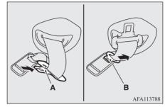
3. Pull the seat belt out slowly and pass it through the seat belt guide (E) so that the latch plate (A) is turned to the front side.
