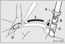
6. Pull the belt slightly to adjust slackness as desired.
