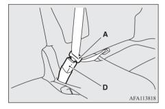
2. To release the buckle (C), press the button (F) with the latch plate (A).
