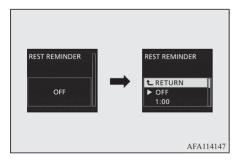
3. Press the ✓ switch or ∧ switch to select the time, and then press the © switch to confirm the setting. The setting is changed to the selected time.
