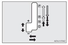
The lock button must be pushed while the brake pedal is depressed to move the selector lever.
