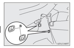
1. Move one of the sliders (C) towards the inside of the vehicle, and fit the tab (D) into the installation hole that is to be used. Move the opposite slider in the same fashion.
