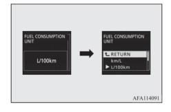
3. Press the ∨ switch or ∧ switch to select the units, and then press the □ switch to confirm the setting.
