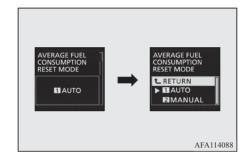
3. Press the \switch or \states switch to select the reset mode, and then press the \sigma switch to confirm the setting.
