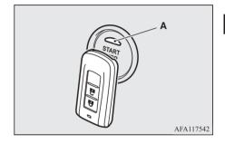
3. If the keyless operation key is recognized, the indication lamp (A) on the engine switch illuminates in green, and then the engine can be started and the operation mode can be changed within approximately 10 seconds. Refer to "Starting the engine" on page 6-20 and "Changing the operation mode" on page 6-16.
