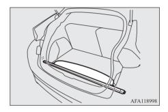
Except for vehicles equipped with a spare tyre, the cover can be stored under the luggage floor board.
