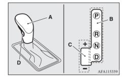
In the main gate, the selector lever has four positions, and is equipped with a lock button (D) to avoid inadvertent selection of the wrong gear.
