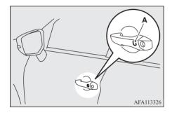
A- Driver's or front passenger's door lock/unlock switch
