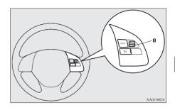
To slow down your speed in small amounts, push down the "SET -" switch (B) for less than approximately 1 second and release it. Each time you push down the "SET -" switch (B), your vehicle will slow down by approximately 1.6 km/h (1 mph).
