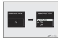
3. Press the ∨ switch or ∧ switch to select the sound, and then press the □ switch to confirm the setting.
