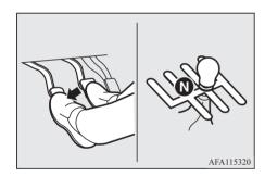
3. Release the clutch pedal. The engine will stop automatically.
