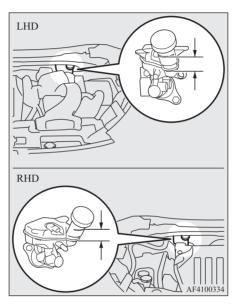
The fluid level is monitored by a float. When the fluid level falls below the "MIN" mark, the brake warning lamp lights up.
