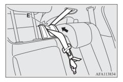
4. After the seat belt is retracted completely, insert the small latch plate (B) into the upper slit (G) and the latch plate (A) into the lower slit (H).
