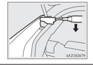
3. Turn the rear turn-signal lamp socket anticlockwise and remove it, and then pull the bulb out of the socket.
