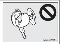
In cases like these, remove the object or additional key from the vehicle key. Then try again to start the engine. If the engine does not start, we recommend you to contact your MITSUBISHI MOTORS Authorized Service Point.
