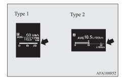
When the value of momentary fuel consumption surpasses the value of average fuel consumption, the momentary fuel consumption is displayed with a white bar graph. (Type 2)
