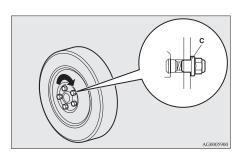
Initially tighten the wheel nuts until the tapered area (A) of the nuts lightly touches the wheel hole seat area (B) enough to keep the tyre from wobbling.
