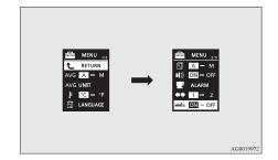
3 Press and hold the multi-information meter switch for about 2 seconds or more to switch in sequence from ON (with the green bar graph)  $\rightarrow$  OFF (without the green bar graph)  $\rightarrow$  ON (with the green bar graph).
