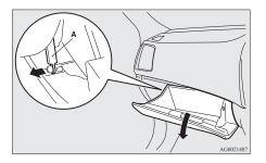
While pressing the side of the glove box, unhook the left and right hooks (B) and lower the glove box.
