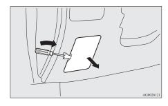
To put back the fuse lid, line up the fuse lid hook (A) with the clamp (B) on the instrument panel and push the lid back in.
