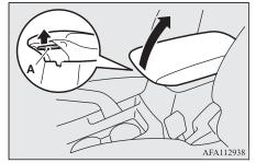
The tissue holder and pen holder are located on the underside of the floor console box lid.
