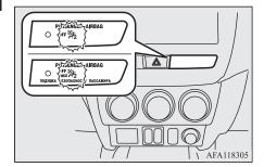
The indicator normally illuminates when the ignition switch is turned to the "ON" position or the operation mode is put in ON, and goes off a few seconds later.
