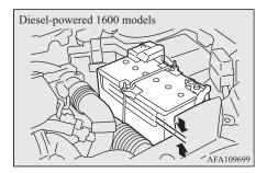
The electrolyte level must be between the specified limit on the outside of the battery. Replenish with distilled water as necessary.
