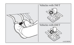
Release the clutch pedal. The "sse" display/indicator will turn on and the engine will stop automatically.
