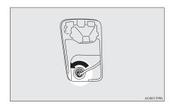
4. Remove the bulb by pulling it out.
