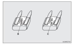
B- Fuse is OK C- Blown fuse
