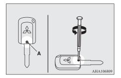
2. With the MITSUBISHI mark facing you, insert the cloth-covered tip of a straight blade (or minus) screwdriver into the notch in the remote control switch case and use it to open the case.
