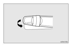
4. The headlamps will come on in the low beam setting for about 30 seconds. After the headlamps go off, the headlamps can be turned on again in the low beam setting for about 30 seconds by pulling the turn signal lever towards you within 60 seconds of turning the ignition switch to the "LOCK" position or putting the operation mode in OFF.
