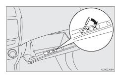
• There is a limit to the size of pens that can be stored in the holder. Forcibly inserting large pens could damage the holder.
