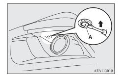
Insert a straight blade (or minus) screwdriver with a cloth over its tip into the fog lamp cover (B) and pry gently to remove it.
