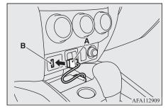
4. To remove the connector cable, turn the ignition switch to the "LOCK" position or put the operation mode in OFF first and perform the installation steps in reverse.
