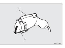
7. Connect the normal charge connector until a click sound is heard without pressing the release button (G).
