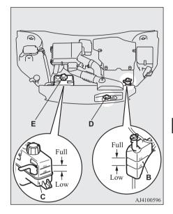
B: Reserve tank for engine cooling C: Reserve tank for EV cooling system
