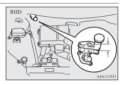
The fluid level is monitored by a float. When the fluid level falls below the "MIN" mark, the brake fluid warning lamp lights up. The fluid level falls slightly with wear of the brake pads, but this does not indicate any abnormality.
