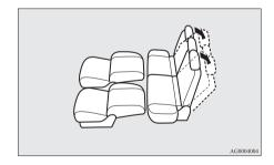
4. The flat seat configuration is now complete. Reverse the above procedures when returning the seat to the normal position.
