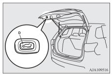
If the close switch on the inside of the electric tailgate is pressed, the electric tailgate closes after the warning buzzer sounds and the hazard warning flasher blinks.
