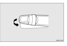
4. The headlamps will come on in the low beam setting for about 30 seconds. After the headlamps go off, the headlamps can be turned on again in the low beam setting for about 30 seconds by pulling the turn signal lever towards you within 60 seconds of putting the operation mode in OFF.
