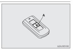
The settings mode can be toggled by pressing the UNLOCK switch. The mode can be confirmed from the number of times the buzzer sounds.
