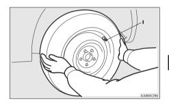
7. Turn the wheel nuts clockwise by hand to initially tighten them.
