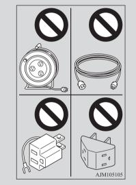
• Do not use a multi type outlet to prevent an electric shock or fire. There is no guarantee of safety because you cannot make an earth connection in some multi type outlet and it is not a dedicated type outlet.
