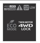
If the ECO mode switch is switched OFF, the drive mode will be returned to "4WD LOCK" mode.
