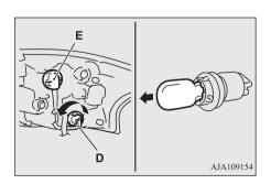
E- Tail lamp and stop lamp (LED)-cannot be replaced
