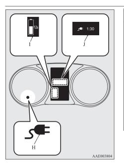
If the charging indicator is not illuminated, charging has not started. Make sure that the normal charge port and the plug are correctly connected, and perform charging from Step 5 again.
