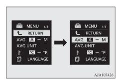
3. Press and hold the multi information display switch for about 2 seconds or more to switch from A/1 (Auto reset mode) to M/2/P (Manual reset mode), or from M/2/P to A/1
