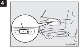
If the open switch is pressed with the tailgate and all doors are unlocked, the electric tailgate opens after the warning buzzer sounds. When the tailgate and all doors are locked, the warning buzzer will not sound.
