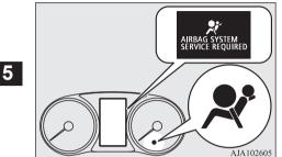
There is a Supplemental Restraint System ("SRS") warning lamp on the instrument panel. The system checks itself every time the operation mode of the power switch is put in ON. The SRS warning lamp will come on for several seconds and then go out. This is normal and means the system is working properly.
