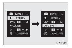
3. Press and hold the multi information display switch for about 2 seconds or more to display "AVG UNIT".
