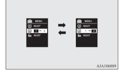
4. The valid tyre ID set is changed, and the number of the tyre pressure monitoring system (TPMS) SET indicator is changed.
