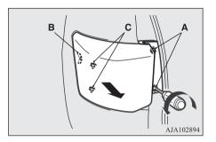
3. Turn the socket anticlockwise and remove it, and then pull the bulb out of the socket.
