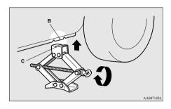
4. Check that the flange portion at the jacking point fits in the groove at the top of the jack.
