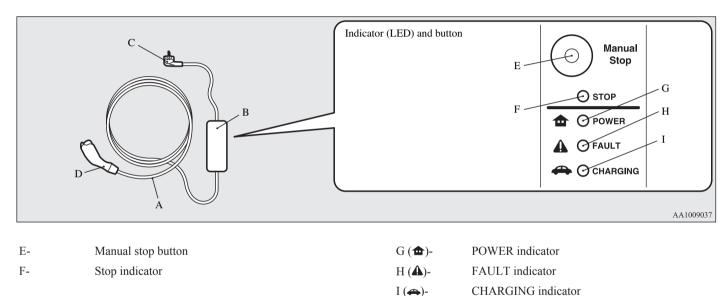
To stop charging, simply press manual stop button (E) and stop indicator (F) is illuminated. Re-connect the EV charging cable plug (C) to charge again.
