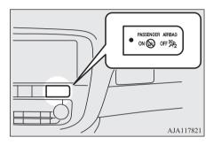
The both indicator normally comes on when the operation mode of the power switch is put in ON, and goes off a few seconds later.
