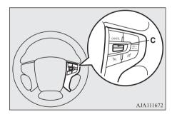
The set speed is increased each about 5 km/h (3 mph) per about 0.5 second.
