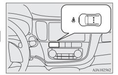
If the operation mode of the power switch is put in ON while a seat belt is not fastened, the warning lamp comes on for approximately 30 seconds to remind the rear passenger to fasten the seat belt.
