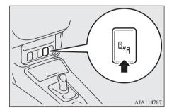
If you turn the BSW ON/OFF, the Rear Cross Traffic Alert (RCTA) also turns ON/OFF at the same time.
