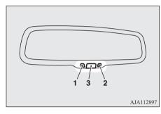
When the operation mode of the power switch is put in ON, the green indicator (1) illuminates and the reflection factor of the mirror is automatically changed.
