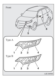
Type A: Halogen headlamps type Type B: LED headlamps type 1- Front turn-signal lamps: 21 W (PY21W) 2- Headlamps, high-beam: 60 W (HB3) 3- Headlamps, low beam Halogen: 55 W (H7) LED: -
