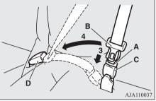
5. Pull the belt slightly to adjust slackness as desired.
