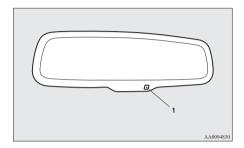
When the operation mode of the power switch is put in ON, the reflection factor of the mirror is automatically changed.
