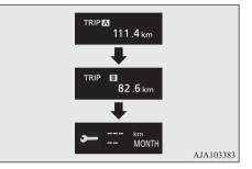
2. Press and hold the multi information display switch for about 2 seconds or more to display "~" and make it flash. (If there is no operation for about 10 seconds with flashing, the display returns to the previous screen.)
