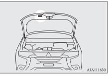
The plate shows the model code, engine model, transaxle model and body colour code, etc.
