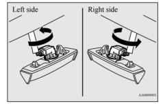
3. Remove the bulb by pulling out.
