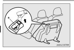
7. Securely retain the second seat by hooking the retaining bands onto the head restraint of the front seat and adjusting the length of the retaining band.
