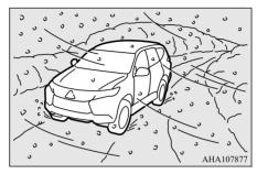
Set the transfer shift lever or the drive modeselector to "4H" position, in accordance with the road conditions, and then gradually depress the accelerator pedal for a smooth start.
