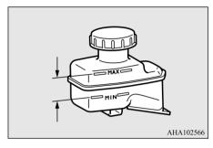
The brake fluid level must be between the "MAX" and "MIN" marks on the reservoir.
