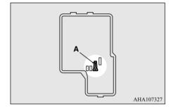
3. Referring to the fuse load capacity table, check the fuse pertaining to the problem.
