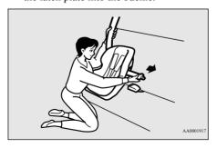
3. To activate the ALR mode, slowly pull the shoulder part of the belt all the way out until it stops, then let the belt feed back into the retractor.
