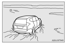
4-wheel drive vehicles are not necessarily waterproof. If the electrical circuits become wet, further operation of the vehicle will be impossible; therefore, avoid crossing streams unless absolutely necessary. If crossing a stream is unavoidable, use the following procedure:
