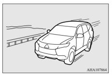
Set the transfer shift lever or the drive modeselector to "2H" or "4H" position to drive on the dry paved road. Especially on dry highway, never select the "4HLc" or "4LLc" position.
