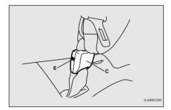
2. After the seat belt is retracted completely, insert the small latch plate (A) into holder (F), and then insert the latch plate (B) into the holder (F).
