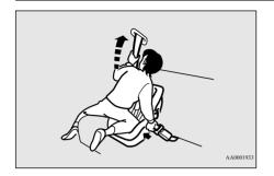
6. Before putting the child in the restraint, push and pull the restraint in all directions to be sure it is secure. Do this before each use. If the child restraint system is not firmly secure, repeat steps 2 through 5.
