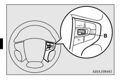
To slow down your speed in small amounts, push down the SET - switch (B) for less than approximately 1 second and release it.
