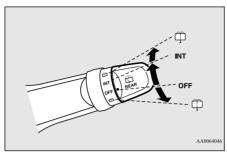
INT - The wiper operates continuously for several seconds then operates intermittently at intervals of approximately every 8 seconds.
