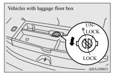
3. Turn the lower cap (C) with the wheel nut wrench, and remove it.
