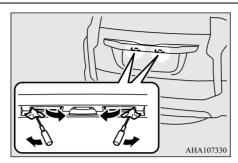
2. Remove the socket and bulb assembly together by turning it anticlockwise.
