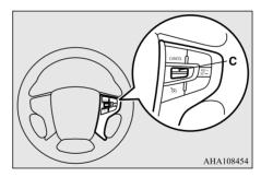
To increase your speed in small amounts, push up the RES + switch (C) for less than approximately 1 second and release it.
