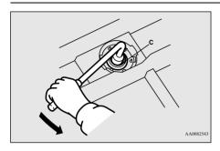
4. Turn the securing bolt (D) anticlockwise with the wheel nut wrench to lower the spare wheel completely to the ground and to slack the chain.
