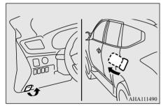
3. Open the fuel tank filler tube by slowly turning the fuel cap anticlockwise.
