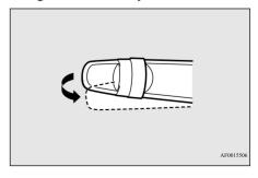
4. The headlamps will come on in the low beam setting for approximately 30 seconds. After the headlamps go off, the headlamps can be turned on again in the low beam setting for approximately 30 seconds by pulling the turn-signal lever towards you within 60 seconds of turning the ignition switch to the "OFF" position or putting the operation mode in OFF.
