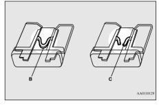
B- Fuse is OK C- Blown fuse
