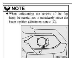
3. Turn the socket anticlockwise to remove it.
