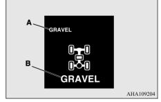
Example: When "GRAVEL" mode is selected The selected control mode is displayed on the Off Road mode indicator display (A).
