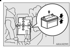
The electrolyte level must be between the specified limit on the outside of the battery. Replenish with distilled water as necessary.
