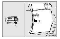
Set the inside lock knob (1) to the locked position, and close the door (2).
