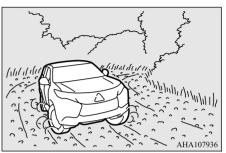
Check the road surface conditions and set the transfer shift lever or the drive mode-selector to "4HLc" or "4LLc". Setting the Off Road mode-selector (if so equipped) to "GRAVEL" may help you drive smoothly.
