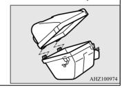
2. Turn the bulb socket anticlockwise to remove it. And remove the bulb from the socket by turning it anticlockwise while pressing in.
