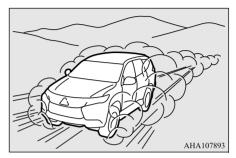
Check the sandy road condition and set the transfer shift lever or the drive mode-selector to "4HLc" or "4LLc". Gradually depress the accelerator pedal to start the vehicle and drive at a possible constant low speed. Either set the Off Road mode-selector (if so equipped) to "SAND", or set the rear differential lock (if so equipped) to ON if the vehicle is likely to get stuck. This may help you drive smoothly.
