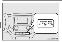
The indicator normally comes on when the ignition switch is turned to the "ON" position or the operation mode is put in ON, and goes off a few seconds later.
