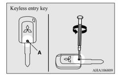
With the MITSUBISHI mark facing you, insert the cloth-covered tip of a straight blade (or minus) screwdriver into the notch in the key case and use it to open the case.
