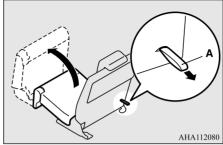
4. Pull the seatback lock release band (B), then tilt the seatback forward until you hear a "click".
