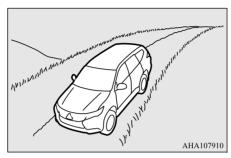
Set the transfer shift lever or the drive modeselector to "4HLc" or "4LLc" position, use the engine brake (downshifting) and descend slowly.
