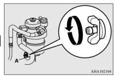
2. Operate the hand pump (B) slowly 6 or 7 times in order to force the water out through the drain plug (A).
