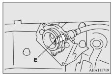
8. Insert the hexagon wrench into the hole where the plug was installed, and continue to turn it anticlockwise while pushing it in.
