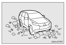
Set the transfer shift lever or the drive mode-selector to "4HLc" or "4LLc" and drive at a low speed. Depending on the road condition, either set the Off Road mode-selector (if so equipped) to "ROCK", or set the rear differential lock (if so equipped) to ON if the vehicle is likely to get stuck. This may help you drive smoothly.
