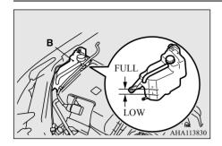
5. Add coolant to the radiator and/or reserve tank if necessary (refer to the "Maintenance" section).
