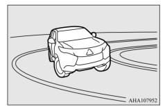
When turning a sharp corner in "4HLc" or "4LLc" position at low speed, a slight difference in steering may be experienced similar to as if the brakes were applied. This is called tight corner braking and results from each of the 4 tyres being at a different distance from the corner.
