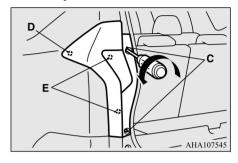
4. Remove each socket and bulb assembly by turning it anticlockwise.
