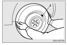
8. Turn the wheel nuts clockwise by hand to initially tighten them.
