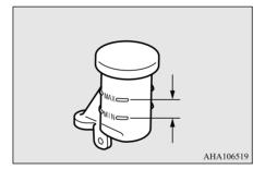
A rapid fluid loss indicates a leak in the clutch system which should be inspected by your authorised MITSUBISHI MOTORS dealer and repaired immediately.
