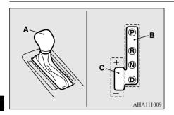
In the main gate, selector lever has 4 positions, and is equipped with a lock button (D) to avoid inadvertent selection of the wrong gear.
