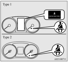
If the ignition switch is turned to the "ON" position or the operation mode is put in ON while the driver's and/or the front passenger's (if so equipped) seat belt is not fastened, the warning lamp comes on and the tone sounds for approximately 6 seconds to remind the driver and/or the front passenger (if so equipped) to fasten the seat belt.
