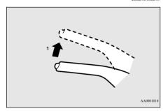
1- Firmly depress and hold the brake pedal, then pull the lever up without pushing the button at the end of hand grip.
