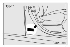
The plate shows model code and engine model, transmission model and body colour code, etc.
