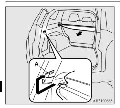
2. Remove the cover from the mounting grooves, and the cover will be rolled back into the retracted position.
