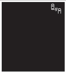
When the BSW switch is pressed again, the indicator on the information screen of the multi-information display will then go out and the BSW will turn off.
