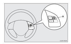
To slow down your speed in small amounts, push down the "SET-" switch (B) for less than approximately 1 second and release it. Each time you push down the "SET-" switch (B), your vehicle will slow down by approximately 1.6 km/h (1 mph).
