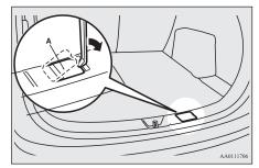
Loosen the tyre hanger installation bolt by turning it anticlockwise with the wheel nut wrench.
