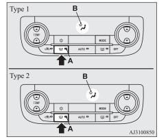
● When the demister switch is pressed, the air conditioning system automatically operates and outside air (as opposed to recirculated air) is selected. This automatic switching control is carried out to prevent misting of the windows even if "Disable automatic air conditioning control" or "Disable automatic air selection control" is set. (Refer to "Customizing the air conditioning switch" on page 7-10, "Customizing the air selection" on page 7-09.)
