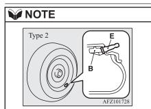
The spare tyre with aluminium wheel has the tyre inflation pressure sensor, so it can be used for tyre rotation.
