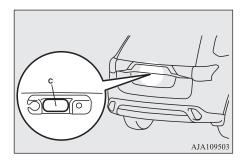
If the open switch is pressed with the tailgate and all doors are unlocked, the electric tailgate opens after the warning buzzer sounds. When the tailgate and all doors are locked, the warning buzzer will not sound.
