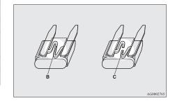
B- Fuse is OK C- Blown fuse
