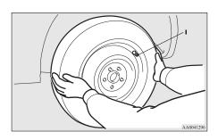
7. Turn the wheel nuts clockwise by hand to initially tighten them.
