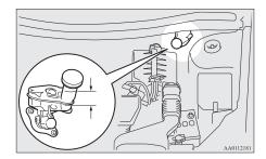
The fluid level is monitored by a float. When the fluid level falls below the "MIN" mark, the brake fluid warning lamp lights up.
