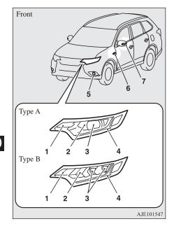
Type A: Halogen headlamps type Type B: LED headlamps type
