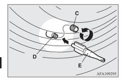
7. Remove the valve insert (F) by turning it anticlockwise using the valve remover (E). Put the removed valve insert in a clean place so it does not get dirty.
