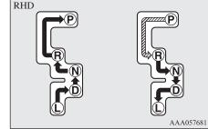
While depressing the brake pedal, move the selector lever through the gate.
