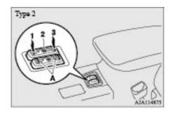
1 (HI) - Heater high (for quick heating).
