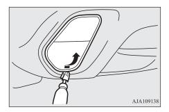
2. Turn the socket (A) anticlockwise to remove it, and then pull the bulb out of the socket.
