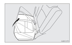
5. Flip the seat cushion forward. On vehicles with the third seats, move the lever (A) to the luggage area mode position.
