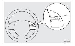
However, the Speed Limiter immediately starts controlling and the vehicle decreases as if an accelerator pedal is closed fully, when the vehicle speed is higher than the set speed.
