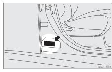
The label shows model code, engine model, transmission model and body colour code, etc.
