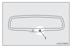
When the ignition switch is turned to the "ON" position or the operation mode is put in ON, the reflection factor of the mirror is automatically changed.
