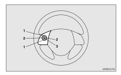
1. ▲ button, ▼ button Adjust audio functions and the mobile phone function volume. 2. < button. > button
