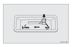
3. While lifting the seat belt's buckle (A), gently lower the seat cushion. Make sure that there is a hook (B) at the position shown in the illustration.
