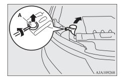
2. Turn the cap (B) anticlockwise to remove it.
