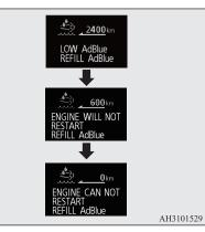
When the driving range is approximately 2,400 km (1,500 miles) or less, a warning display will appear on the information screen in the multi-information display. The warning displays will appear according to the amount of  $AdBlue^{TM}$  remaining.
