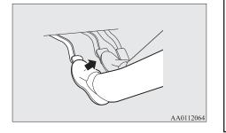
[For vehicles with CVT] 1. Stop the vehicle. 2. Depressing the brake pedal. The engine will stop automatically.
