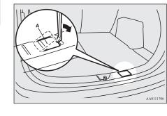
2. Loosen the tyre hanger installation bolt by turning it anticlockwise with the wheel nut wrench.
