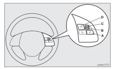
**A-SPEED LIMITER ON/OFF switch** To turn on/off the Speed Limiter.
