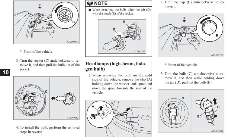
2. Turn the cap (B) anticlockwise to re-
