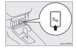
If you turn the BSW ON/OFF, the Rear Cross Traffic Alert (RCTA) also turns ON/OFF at the same time.
