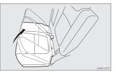
Flip the seat cushion forward. On vehicles with the third seats, move the lever (A) to the luggage area mode position.
