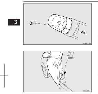
3. Pull the windscreen wiper and washer switch towards you and hold it there. (Since the ignition switch is in the "LOCK" position or the operation mode in OFF, washer fluid will not be sprayed.)
