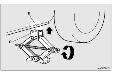
4. Insert the jack bar (D) into the wheel nut wrench (E). Then put the end of the jack bar into the shaft's jack end, as shown in the illustration.
