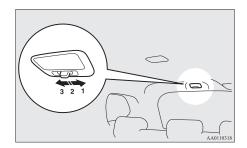
1-  $(\varpi)$ The lamp illuminates regardless of whether the tailgate is open or closed.
