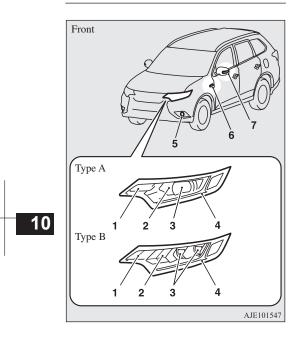
Type A: Halogen headlamps type Type B: LED headlamps type 1- Front turn-signal lamps: 21 W (PY21W) 2- Headlamps, high-beam Halogen: 60 W (HB3) LED: -
