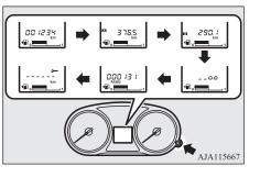
2. Press and hold the multi information display switch for about 2 seconds or more to make the spanner mark start flashing. (If there is no operation for about 10 seconds with flashing, the display will revert to its original indication.) 3. Lightly press the multi information display switch while the icon is flashing to change the display from "---" to "cLEAr". After this, the time until the next periodic inspection will be displayed.
