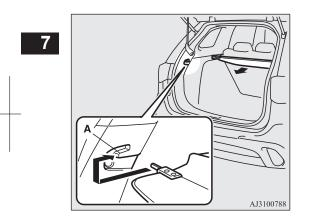
2. Remove the cover from the mounting grooves, and the cover will roll back into the retracted position.
