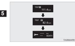
2. Press and hold the multi information display switch for about 2 seconds or more to display "~" and make it flash. (If there is no operation for about 10 seconds with flashing, the display returns to the previous screen.) 3. Lightly press the multi information display switch while the icon is flashing to change the display from "---" to "CLEAR". After this, the time until the next periodic inspection will be displayed.
