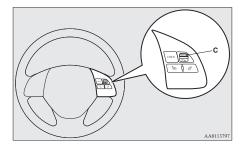
The set speed is increased each approximately 5 km/h (3 mph) per approximately 0.5 second. If a driver wants to increase the set speed a little, push up "RES +" switch for less than approximately 0.5 second and release it. The set speed is increased 1 km/h (1 mph) each taps.
