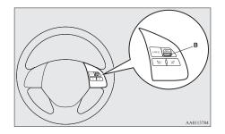
If the current vehicle speed is lower than approximately 30 km/h (19 mph) (settable minimum speed), the set speed is set at approximately 30 km/h (19 mph).
