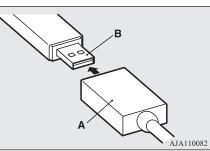
4. Connect the USB connector cable to the USB input terminal.
