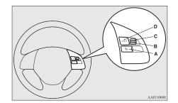
**A- CRUISE CONTROL ON/OFF switch** Used to turn on and off the cruise control.
