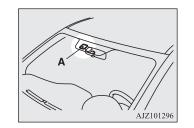
• If the lamps do not turn on or off with the switch in the "AUTO" position, manually operate the switch and we recommend you to have your vehicle checked.
