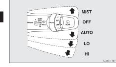
If the lever is put in the "AUTO" position, the rain sensor (A) will detect the extent of rain (or snow, other moisture, dust, etc.) and the wipers will operate automatically. Keep the lever in the "OFF" position if the windscreen is dirty and the weather is dry. Wiper operation under these conditions can scratch the windscreen and damage the wipers.
