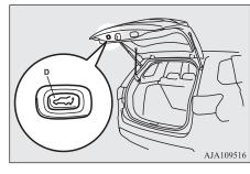
If the close switch on the inside of the electric tailgate is pressed, the electric tailgate closes after the warning buzzer sounds. If the close switch is pressed once while the tailgate is closing, the warning buzzer sounds and the electric tailgate opens.
