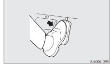
Put on an accelerator pedal to the pedal stroke end. (over a detent that makes pedal reaction force bigger before pedal stroke end)
