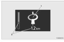
1- Guidance display Shows the direction of vehicle travel and the guidance location. **NOTE**
