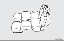
5. The flat seat configuration is now complete. Reverse the above procedures when returning the seat to the normal position.
