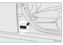
The label shows model code, engine model, transmission model and body colour code, etc.
