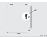
3. Referring to the fuse load capacity table, check the fuse pertaining to the problem.
