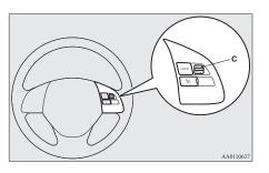
To increase your speed in small amounts, push up the "RES+" switch (C) for less than approximately 1 second and release it.
