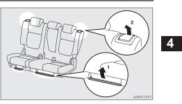
1- To adjust forward or backward (vehicles with second seat slide function) Lift the handle and adjust the seat to the desired position, and release the handle.
