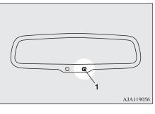
When the ignition switch is turned to the "ON" position or the operation mode is put in ON, the reflection factor of the mirror is automatically changed.
