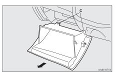
When changing the fuse of the sub fuse block, perform it with the hole of the bottom cover.
