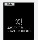
Have an inspection made by a MITSUBISHI MOTORS Authorized Service Point. For vehicles equipped with mono-colour liquid crystal display meter, drive mode indicator ("4WD-E", "LOCK") is blinking at the same time.
