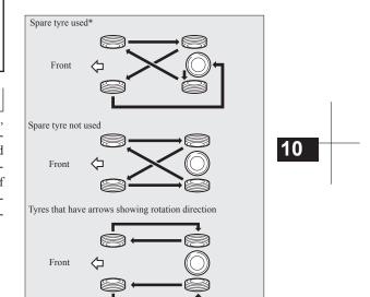
\*: If the spare tyre wheel differs from the standard tyre wheel, do not perform tyre rotation using a spare wheel.
