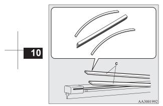
4. Insert the wiper blade into the arm, starting with the opposite end of the blade from the stopper. Make sure the hook (B) is fitted correctly in the grooves in the blade.
