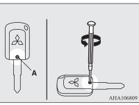
3. With the MITSUBISHI mark facing you, insert the cloth-covered tip of a straight blade (or minus) screwdriver into the notch in the remote control switch case and use it to open the case.
