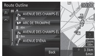
This displays a list of junctions at which turns must be made.
