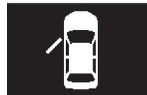
If any of the doors or the tailgate is not completely closed, this displays the open door or tailgate.
