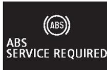
If there is a malfunction in the system, the ABS warning lamp will come on and the warning display will appear on the information screen in the multi-information display. Under normal conditions, the ABS warning lamp only comes on when the ignition switch is turned to the “ON” position or the operation mode is put in ON and goes off a few seconds later.
