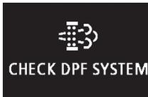
If an abnormal condition occurs in the DPF system, the DPF warning display and check engine warning lamp illuminate. Have the system inspected by a MITSUBISHI MOTORS Authorized Service Point.
