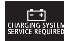
If there is a fault with the charging system, the warning display is displayed on the information screen in the multi-information display. The warning lamp in the instrument cluster also illuminates.
