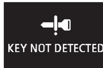
When the vehicle is parked with the operation mode in any mode other than OFF, if you close the door after opening any of the doors and taking the keyless operation key out of the vehicle, a warning displays and the buzzer sounds 4 times.
