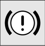
This lamp illuminates when the ignition switch is turned to the “ON” position or the operation mode is put in ON, and goes off after a few seconds.
