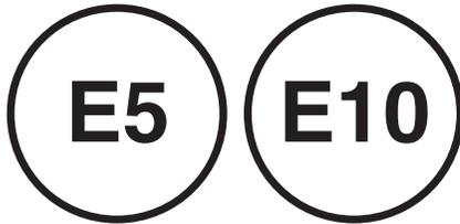
E5: Petrol fuel containing up to 2.7 % (m/m) oxygen or up to 5.0 % (V/V) ethanol – Eg. EN 228 compliant unleaded petrol
