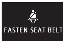
A tone and warning lamp are used to remind the driver to fasten the seat belt.
