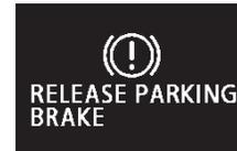
This warning is displayed if you drive with the parking brake still applied. The warning lamp in the instrument cluster only illuminates when the parking brake is applied.
