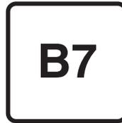
B7: Diesel fuel containing up to 7.0 % (V/V) Fatty Acid Methyl Esters – Eg. EN 590 compliant diesel
