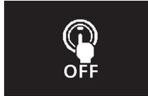
If the driver’s door is opened with the engine stopped and the operation mode in any position other than OFF, the operation mode ON reminder buzzer sounds intermittently to remind you to put the operation mode in OFF. In addition, the warning display will be displayed on the information screen in the multi-information display.
