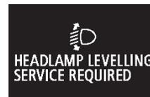
If there is a fault in the automatic headlamp levelling system, the warning display is displayed on the information screen in the multi-information display.
