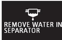
When the ignition switch is turned to the "ON" position or the operation mode is put in ON, if more water than the specified limit has accumulated in the fuel filter, the warning display is displayed on the information screen in the multi-information display.
