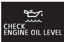
When the ignition switch or the operation mode is in ON, if it is suspected that the engine oil level has increased excessively, the warning display is displayed on the information screen in the multi-information display.
