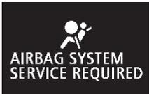
The system checks itself every time the ignition switch is turned to the "ON" position or the operation mode is put in ON. The SRS warning lamp will come on for several seconds and then go out. This is normal and means the system is working properly.
