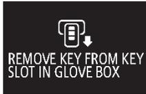
If the operation mode is in OFF and the driver's door is opened with the keyless operation key in the key slot, a warning is issued with the warning display and the buzzer buzzing for approximately 3 seconds to remind you to remove the key.
