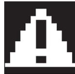
This is displayed when you press the multi-information meter switch and switch the warning display screen.
