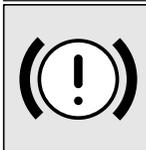
This lamp illuminates when the ignition switch is turned to the “ON” position or the operation mode is put in ON, and goes off after a few seconds.
