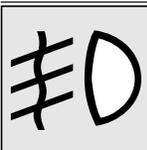
This lamp illuminates while the front fog lamps are on.
