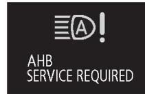
[When the sensor is malfunctioning]
