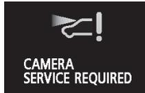
If the message remains even after the ignition switch is turned to the “LOCK” position and then turned back to the “ON” position or the operation mode is put in OFF, and then turned back to “ON”, please contact a MITSUBISHI MOTORS Authorized Service Point.
